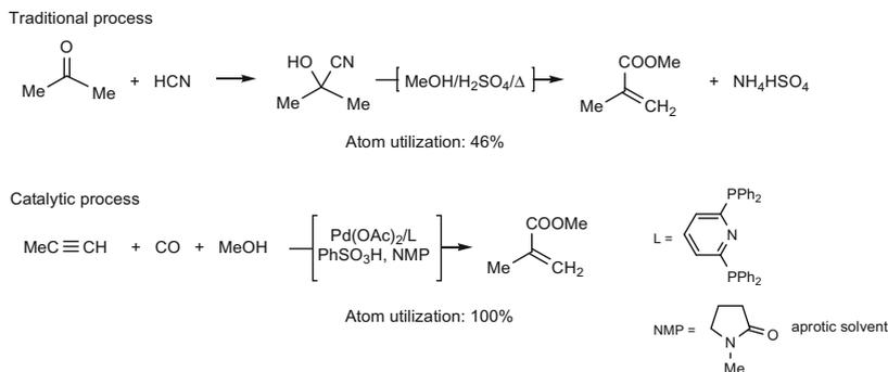
**Scheme 1.19** Traditional and catalytic process for the production of methyl methacrylate
