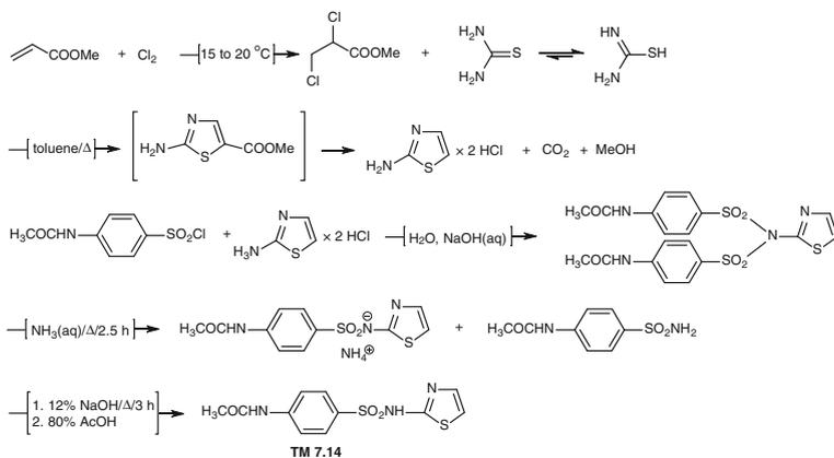
**Scheme 7.21** Industrial method for production of *sulfathiazole* **TM 7.14**
