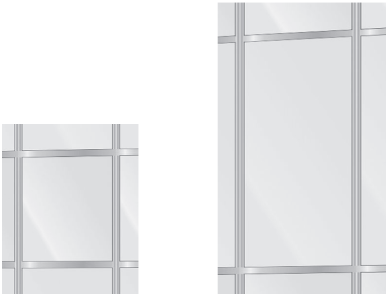
Fig. 5-2. Example vision openings: (left) 1200 mm \times 1200 mm vision opening; (right) 1500 mm \times 2750 mm vision opening Source: Sota Glazing, Inc.
