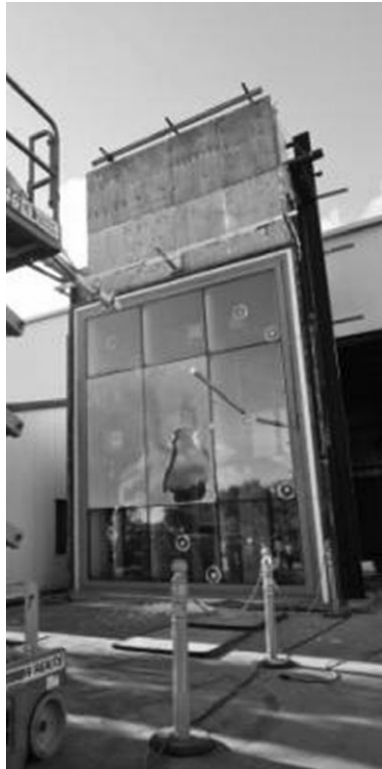
Fig. 4-12. Example of large frame curtain wall with missile (wood 2x4 stud) Source: Courtesy of Architectural Testing Inc.; reproduced with permission
