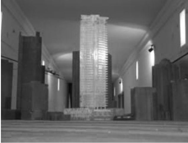
Fig. 4-17. Scaled building model in wind tunnel test Source: Courtesy of CPP, Inc.; reproduced with permission
