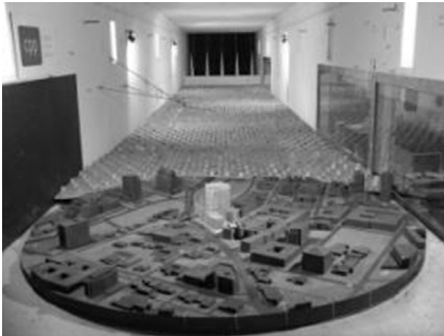
Fig. 4-18. Wind tunnel testing Source: Courtesy of CPP, Inc.; reproduced with permission
