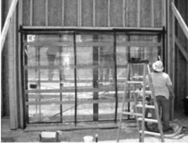
Fig. 4-13. A representative box chamber around a specimen that tests air leakage and water infiltration
