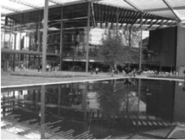
Fig. 3-1. Winspear Opera House, Dallas, TX; an example of all clear glazed façade
