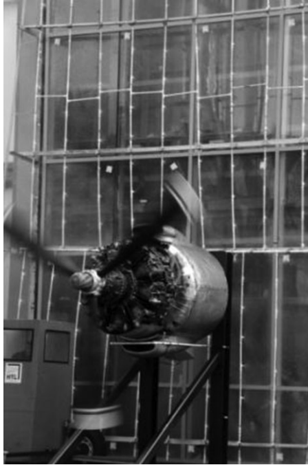
Fig. 4-6. Representative mockups for dynamic water testing at laboratory Source: Courtesy of Architectural Testing Inc.; reproduced with permission
