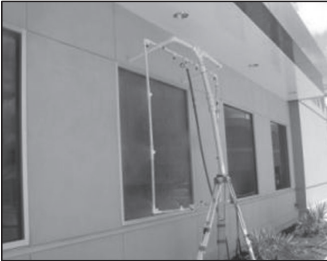
Fig. 4-16. A spray rack test AAMA 503
