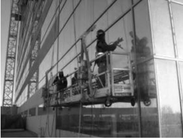
Fig. 4-15. A hose nozzle test AAMA 501.2
