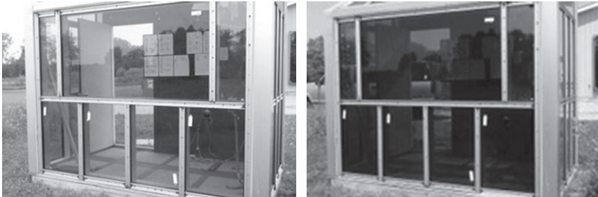
Fig. 10-14. Nonactivated (left) versus activated (right) thermo-chromic glass (Pleotint 2013)
