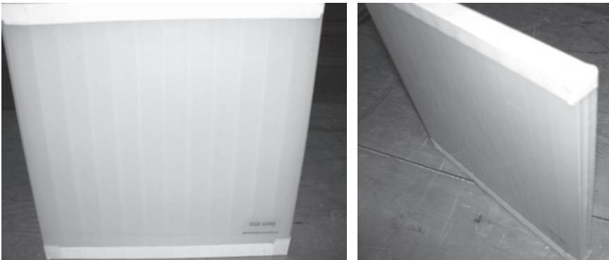
Fig. 11-9. Sample of multiwall polycarbonate sheet filled with aerogel
