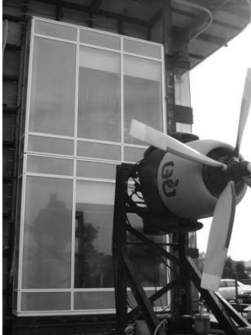
Fig. 4-2. Example of an installed two-story mockup for testing Source: Courtesy of Construction Consulting International; reproduced with permission
