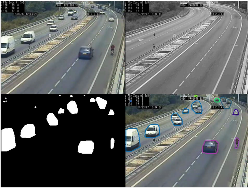
Fig. 3 Frame 269 processed by the proposed method. The blob corresponding to the cyclist is old enough to appear in the segmented image.
