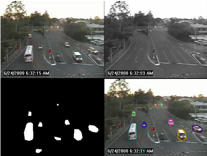
Fig. 4 Frame 204 processed by the proposed method. One of the cars stopped at the traffic light has not been tagged in the segmented image. The colour of the car is too similar to the colour of the road. Although a blob corresponding to the front of this car can be seen on the bottom left image, it is too recent as no blob was detected for this car on the previous frame.
