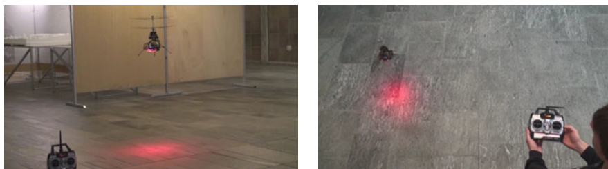
Fig. 8 CoaX helicopter in a velocity control experiment: hovering (left) and following a square path (right)
