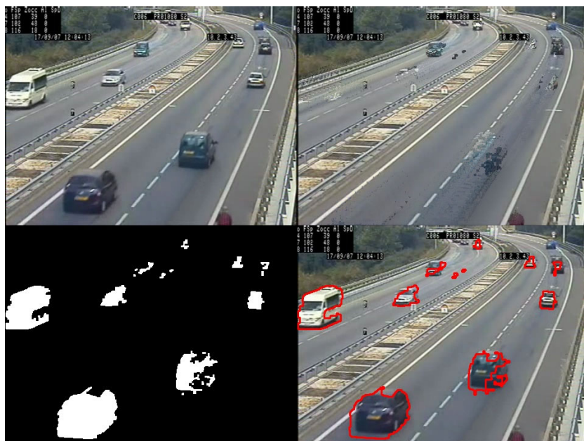
Fig. 6 Frame 68 processed by the OpenCV library method. The cyclist is missing from the binary image. Slow moving objects smear the model image.
