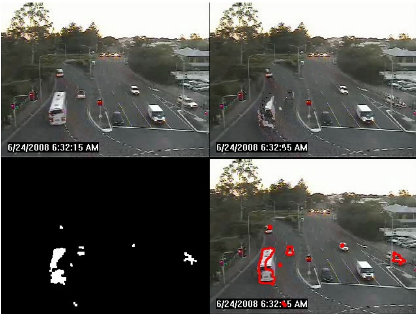
Fig. 8 Frame 204 processed by the OpenCV library method. When cars slow down at the traffic light, they become part of the background.
