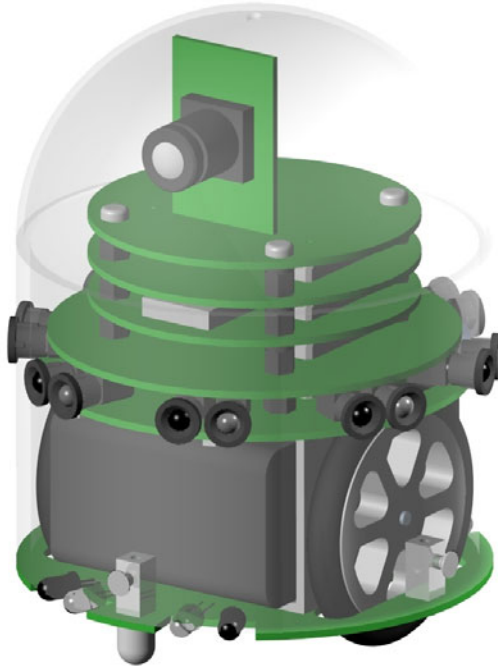
Fig. 1 See through view of the AMiRo robot showing the stackable modules (CAD drawing)
