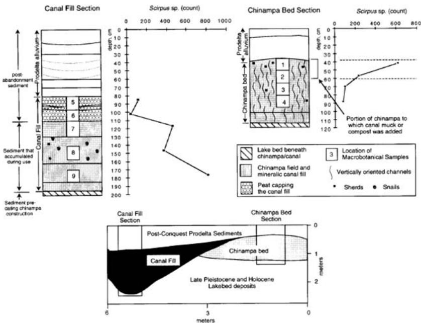
**Figure 5.** Trends in bulrush (*Scirpus* sp.) from the Ayotzingo *chinampa* and canal (Frederick 1997; unpublished data). Bulrush would have been growing in the canal when the *chinampa* was first constructed, and the concentration of bulrush seeds at the top of the *chinampa* field is best explained by either mucking (dredging of mud from the canal and placing it on the ridge) or addition of compost containing Bulrush.
