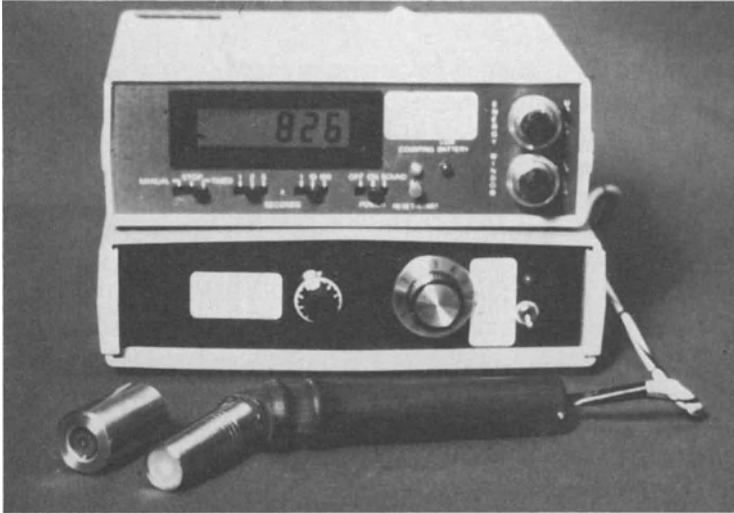
Figure 5. Improvements in the gamma detecting probe included a 1-cm crystal, a modified pre-amplifier concealed in the handle, and amplified sound.
