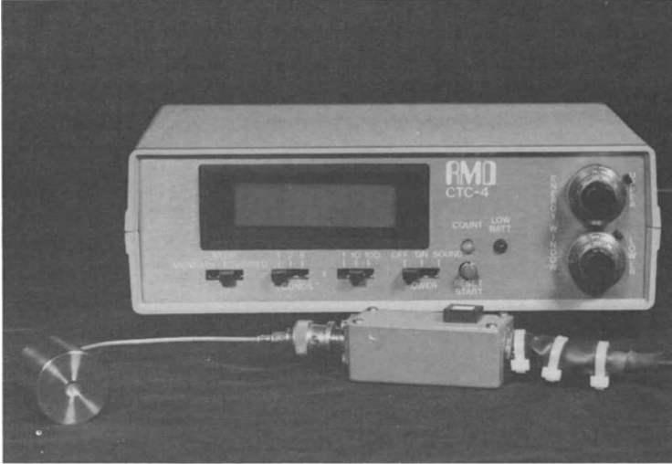
Figure 1. The first gamma detecting probe consisted of a cadmium telluride crystal, preamplifier, and a digital read-out display.
