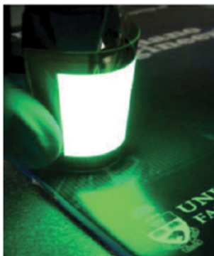
FIGURE 2.5 (a) Schematic of the OLED device structure on low-cost flexible plastic with metal electrodes. (b) Photograph of a large-area flexible OLED (50×50 mm 2 ) working at high luminance (>5000 cd/m 2 ). [Source: Wang et al. [48], Figure 1, p. 754. Adapted with permission from Nature Publishing Group.]
