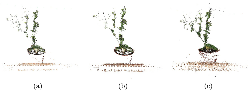
Fig. 2. Sparse 3D point clouds (keypoints) by different feature algorithms in SFM from 75 images of an Arabidopsis. (a) 16340 keypoints by SURF/SIFT. (b) 56784 keypoints by Akaze. (c) 33335 keypoints by DAISY.
