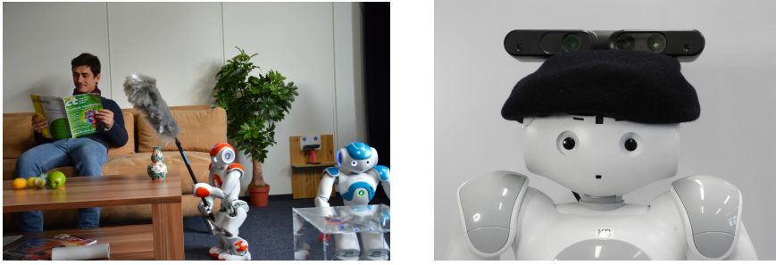
Fig. 1. (Left) Final scenario to be used and (Right) NAO robot with RGB-D device
