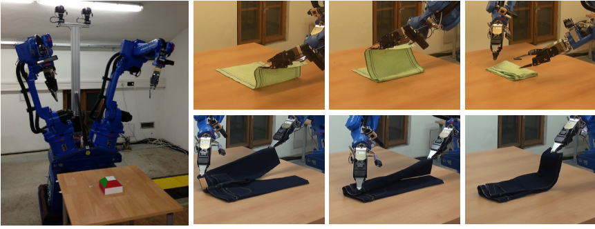
Fig. 1. Our robotic test platform utilizes two industrial hollow-wrist welding manipulators Motoman MA1400 with mounted cameras, Kinect-like rangefinders and dedicated grippers. We use it as the experimental platform for folding of various types of clothes.
