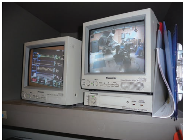
Figure 21.8 Monitoring from immediately outside the treatment room is accomplished with a video screen displaying the child, an intercom system for audio, and a video monitor displaying the electrocardiogram, respiratory wave, and fraction of inspired oxygen. An additional camera allows viewing of the patient simultaneously.
