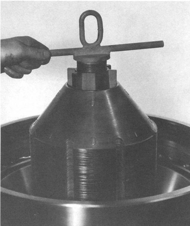
**Figure 4.8c** The rising channel formed by the cut-out at the periphery of the disk, forming a continuous channel for suspension feeding in the disk stack
