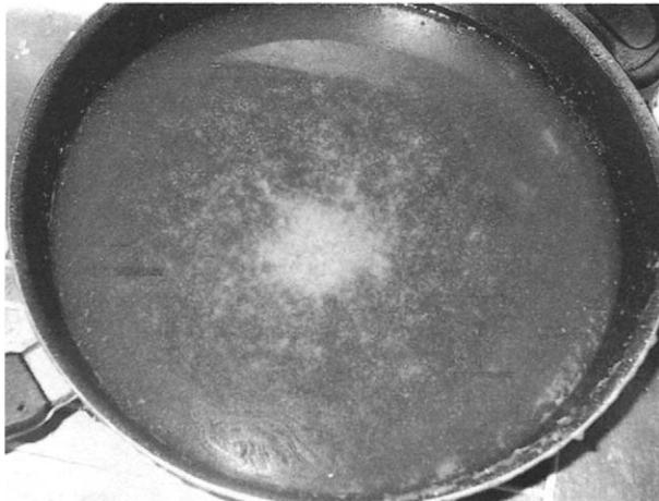
**Figure 2.3c** Photo taken at  $t = 25$  s after stirring stopped, liquid coming to standstill, particulates accumulate near center
