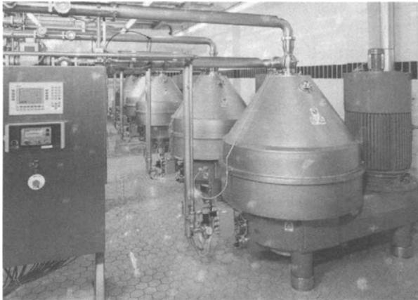
**Figure 4.4** Multiple disk-stack centrifuges in operation (Reproduced by permission of Westfalia Separator)
