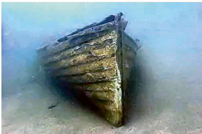
Fig. 14.8 The plumb bow of the motorboat, sports a protective metal bumper band and a one and a half inch metal mooring ring
