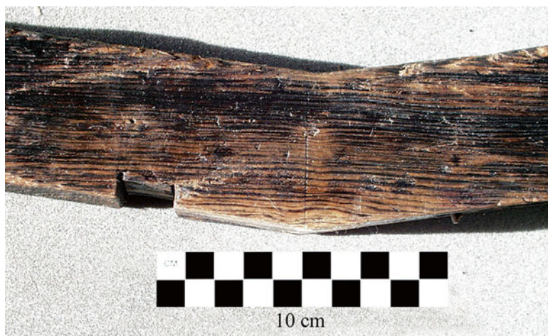
Fig. 6.9 Close-up view of Frame V (forward molded surface) showing the limber hole and the scribe mark denoting the centerline
