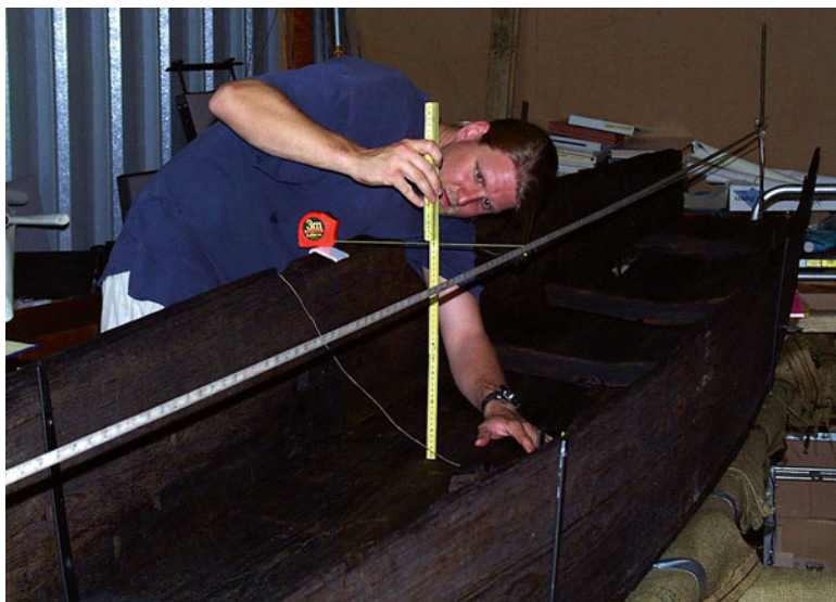
Fig. 6.5 The author recording the interior curvature of the hull at the midships body station, or the widest point of the vessel (located 2.46 m forward of the stern, which is in background of photograph)
