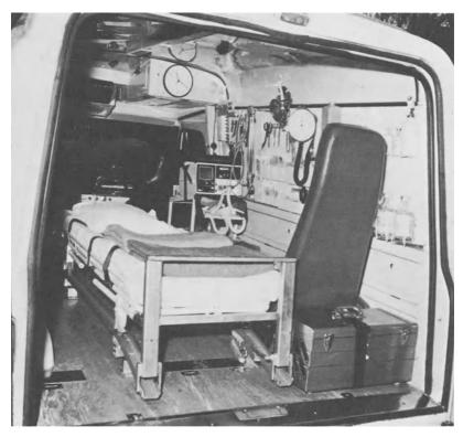
Fig. 3-1. Interior of Melbourne Mobile Intensive Care Units showing portable monitor, defibrillator, and drug box.
