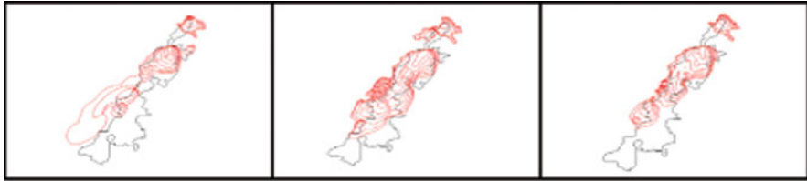
Fig. 3 Simulation of FARSITE for the fire in Rafina on 28-07-2005 for the tests 1, 2 and 3 of fuel models. The black line is the real burnt land whereas the red line shows the simulated burnt land of the fire per hour
