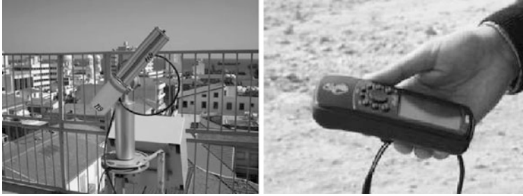
Fig. 3 CIMEL SUN-PHOTOMETER – hand-held Sun photometer – Microtops II (Cyprus University of Technology Premises-Remote Sensing Lab)
