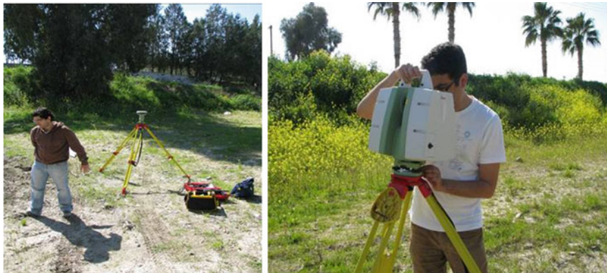
Fig. 3 Rover GPS equipment ( left ). Use of the Leica ScanStation C10 laser scanner in Yialias catchment area ( right )
