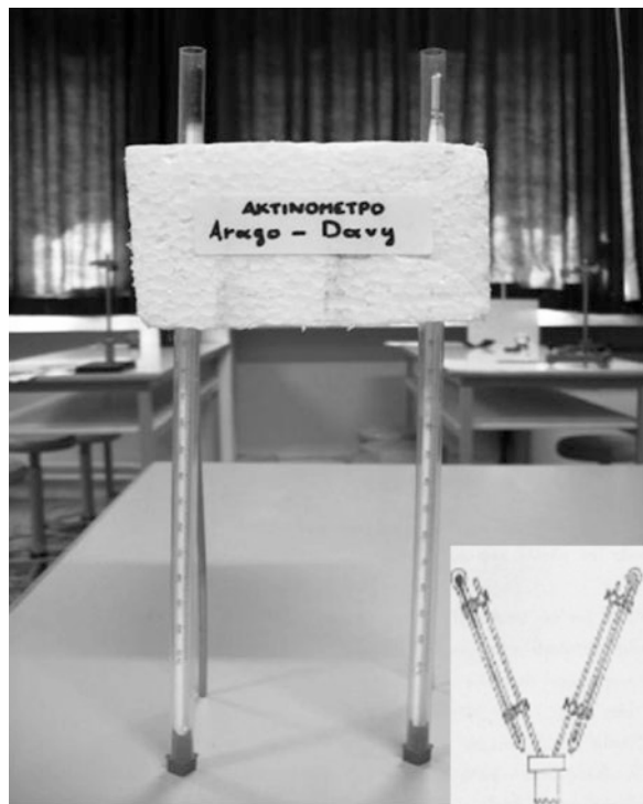
Fig. 1 A reproduction of an Arago-Davy actinometer (Model instrument at lower right )
