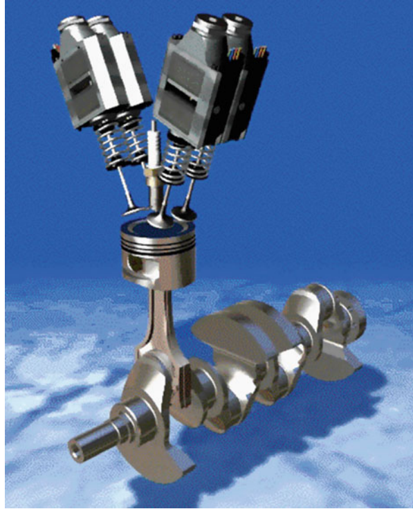
Fig. 2.34 Electromagnetic valves at intake and exhaust
