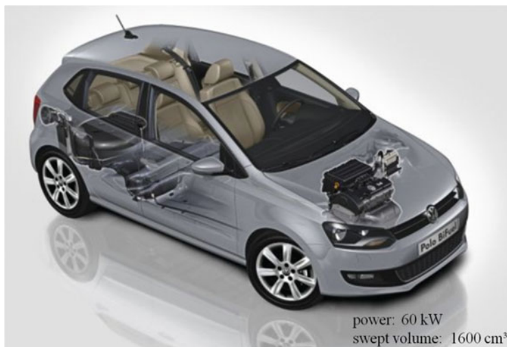
Fig. 3.18 VW Polo bifuel with bivalent operation using LPG and gasoline (Source: Volkswagen)
