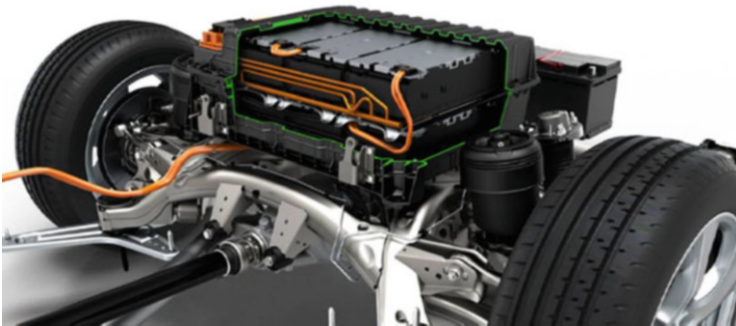
Fig. 5.69 BMW X5 eDrive plug-in hybrid: Li-ion battery (Source: BMW)
