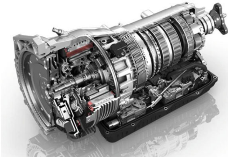
Fig. 5.67 BMW X5 eDrive plug-in hybrid: motor within automatic gear with eight stages (Source: BMW)
