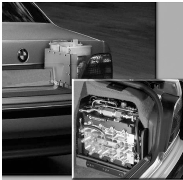
Fig. 3.35 Fuel cell with hydrogen for on-board current generation for an automobile with hydrogen SI engine (Source: BMW)
