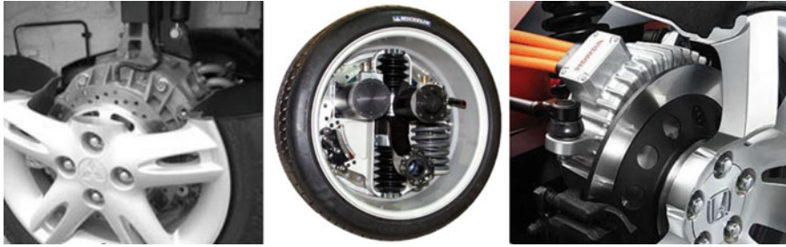
Fig. 5.2 Hub motors for car propulsion: Mitsubishi ( left ), Michelin ( center ), Honda ( right ) (Sources: Mitsubishi, Michelin, Honda)
