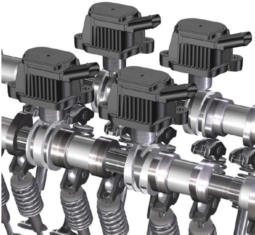
Fig. 2.27 System for shifting of cam profiles (Source: Volkswagen)
