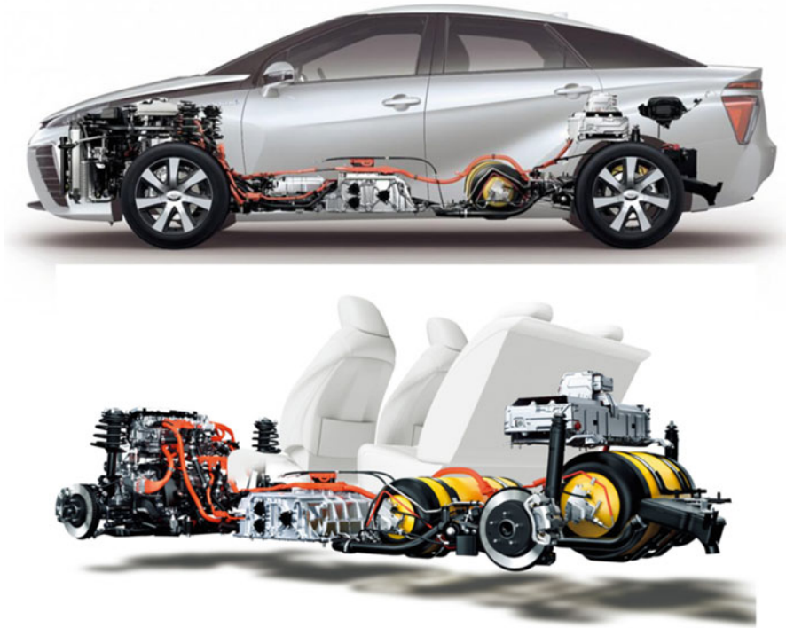
Fig. 4.21 Automobile with electric propulsion using a hydrogen fuel cell (Source: Toyota)
