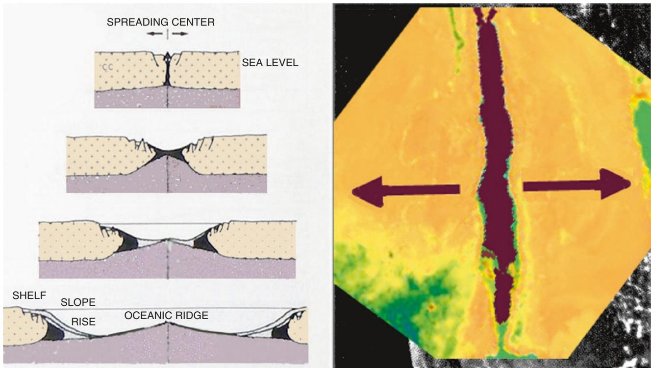
**Fig. 3.5** Evolution of Atlantic-type continental margin. *Left*: sketch of sequence from uplift and expansion of the continental crust and volcanism to accumulation of sediment (stippled) and volcanic deposits (black) to regular seafloor spreading with sinking of the trailing edges.
