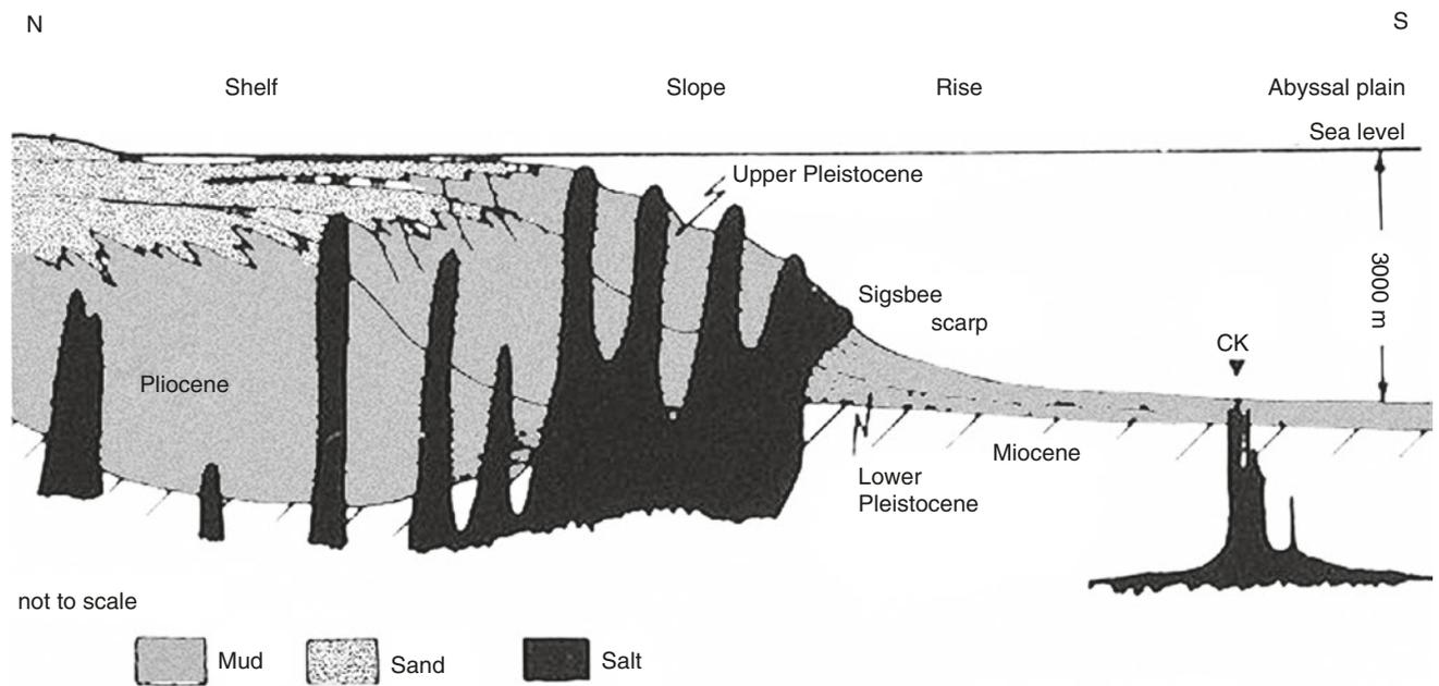
**Fig. 14.4** Salt plumes in the Gulf of Mexico: Mesozoic salt intruding Neogene mud (After C.J. Stuart and C.A. Caughey, 1977, *AAPG Geol. Mem.*, 26, modif.; “CK”, Challenger Knoll, a salt dome below the continental slope (position from DSDP Leg 1))
