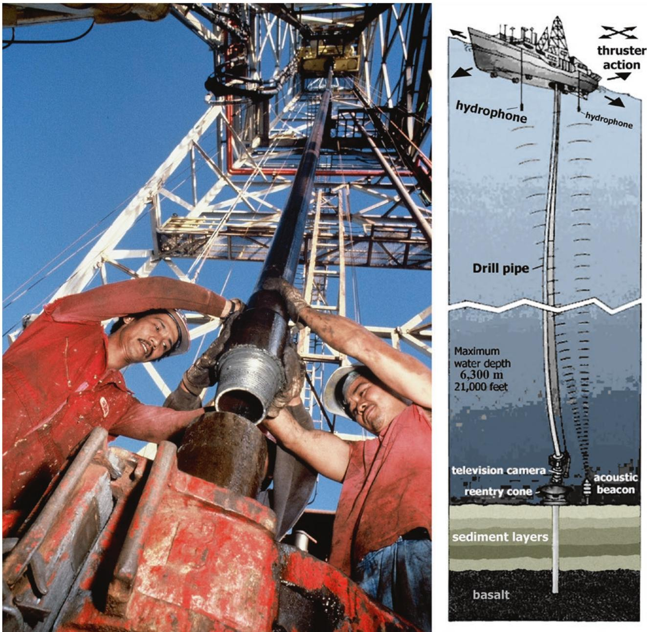
**Fig. 12.5** Retrieving information on Cenozoic history from the seafloor. The chief source of information is drilling from a vessel (here: the JOIDES Resolution is a vessel originally used by BP in commercial
