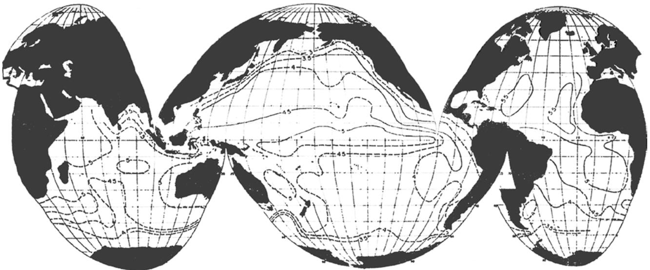
**Fig. 10.10** Topography of the carbonate compensation depth (CCD). The seafloor facies boundary (in places extrapolated) between calcareous sediments and sediments with no or very little carbonate. Numbers:
