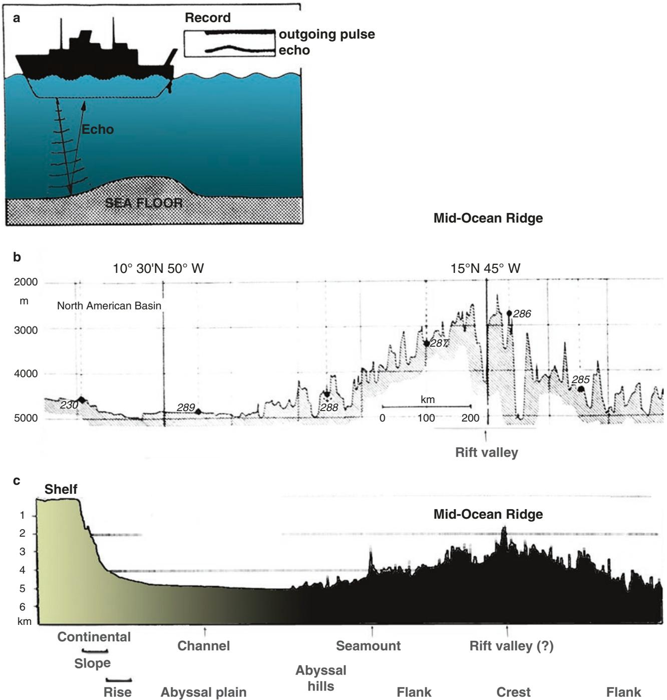
**Fig. 2.2** Topography of the Mid-Atlantic Ridge as observed by echo sounding. (a) The depth emerges from the time it takes the echo to return and the speed of sound in seawater. The two-way travel time is recorded on the sounding vessel (inset: "Record"). (b) Results of echo sounding obtained by the German Meteor Expedition (1925–1927).
