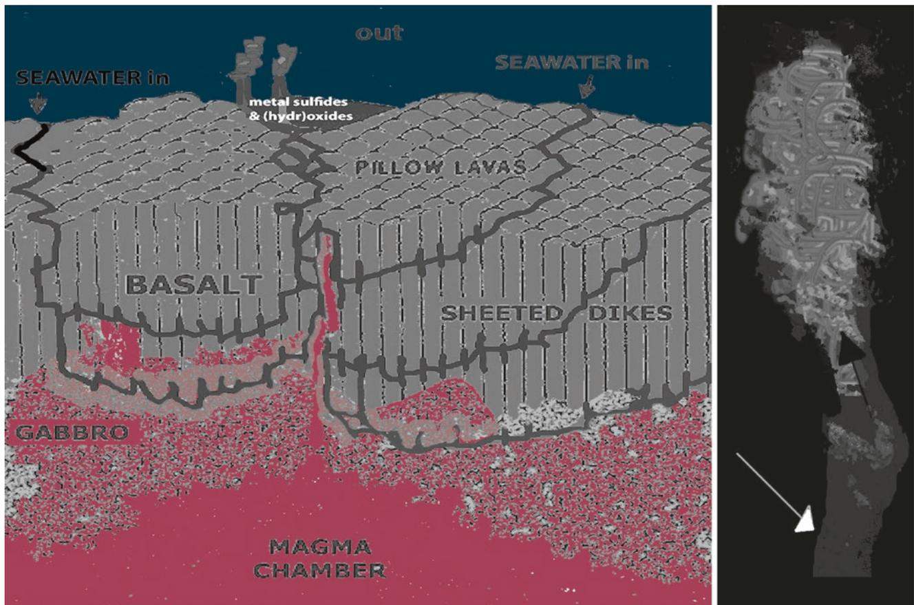
**Fig. 14.13** Black smokers as a resource for metals. The smoker has reaction products of seawater with hot basalt exiting from chimneys (black arrow). Resources are largely sulfide chimneys (white arrow)
