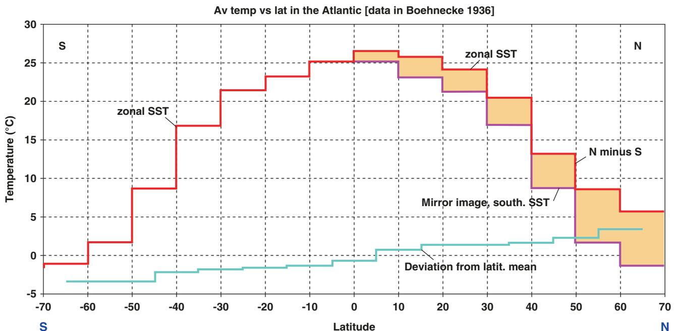
**Fig. 9.7** Temperatures of surface waters in the Atlantic (*heavy red line*) and the amount by which the northern ones exceed the southern ones by latitude (*orange fields*) [Data from G. Boehnecke, 1936, cited in Sverdrup et al., 1942]
