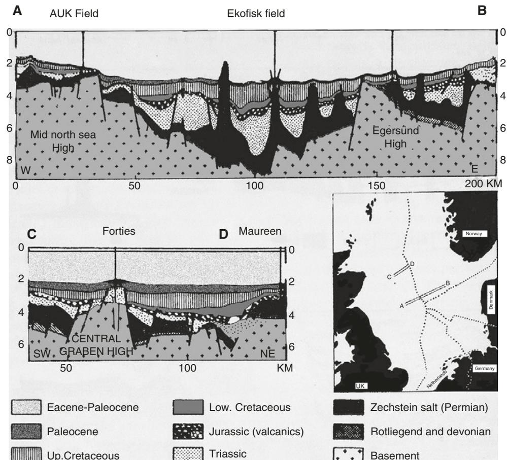
**Fig. 14.5** Geological profiles under the North Sea, with hydrocarbon fields. Vertical exaggeration 6.7x. *Insert:* Map with national shelf boundaries (After P.A. Ziegler, 1977, modified for clarity. See *Geol. Journal* 1:7)
