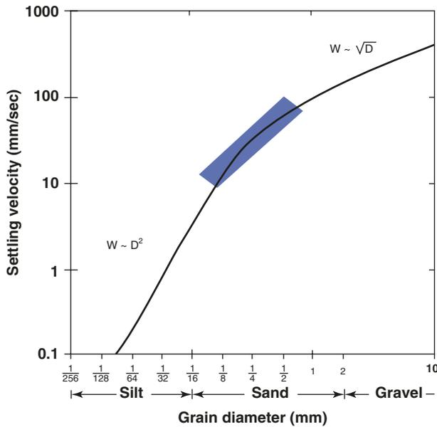
**Fig. 5.5** Settling velocities of quartz grains in water. Silt and fine sand settle according to one equation (velocity a function of square of diameter; Stokes' Law) and coarse sand and gravel according to another (velocity a function of the square root of diameter). The transition zone (blue) is shaded (After W.W. Rubey, 1933, as quoted in C.O. Dunbar and J. Rodgers, 1957. *Principles of Stratigraphy*. John Wiley, New York, modified). Note that sizes are plotted in steps of factor of two
