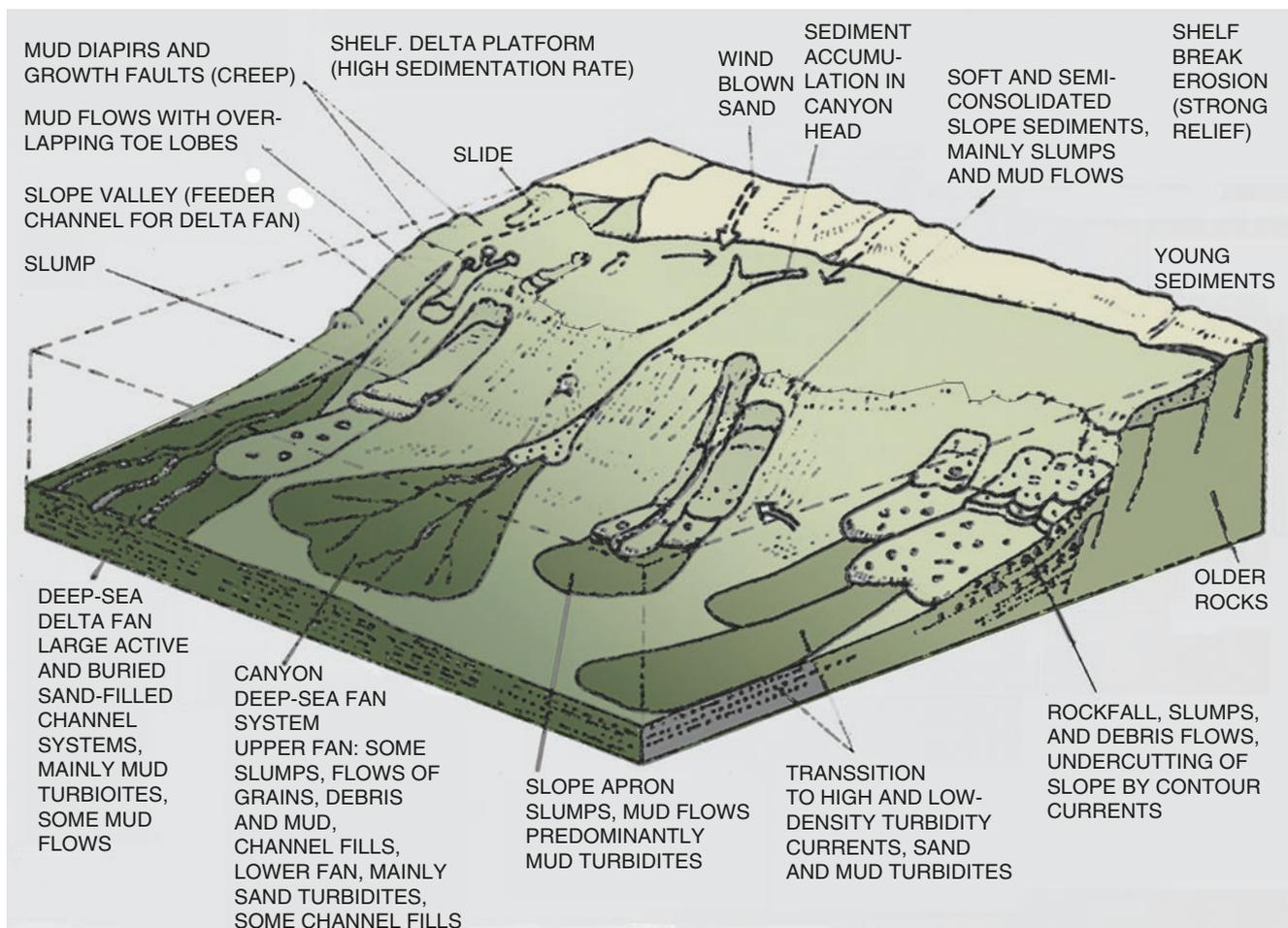
**Fig. 3.15** Sketch of exogenic processes shaping continental margins (G. Einsele in Einsele et al. (eds.) 1991. *Cycles and Events in Stratigraphy*. Springer, Heidelberg) Note the olive-green color of the
