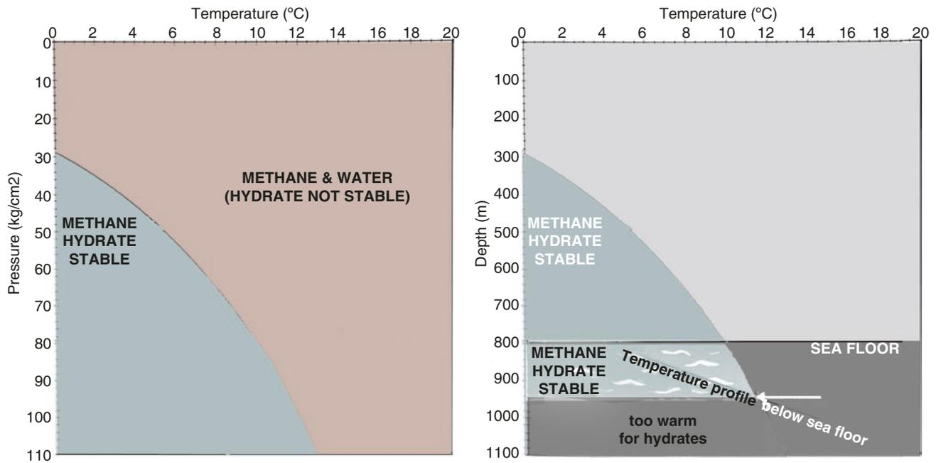
**Fig. 4.5** Stability field of methane ice (*left panel, a*) and application to sedimentary deposits (*right panel, b*). A bottom-simulating reflector (BSR) can occur at the bottom of the layer bearing methane hydrate. At the BSR sound is strongly reflected. The distribution of clathrate is restricted; its presence requires appropriate temperature and pressure to ensure survival if clathrate is present, in addition to a source of methane
