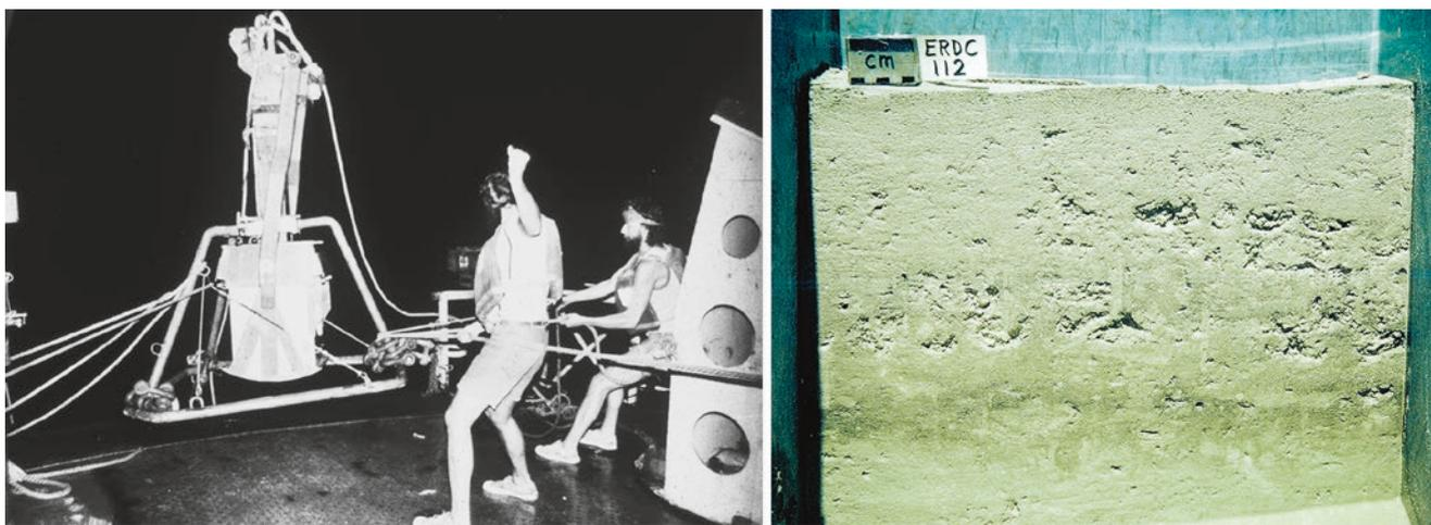
**Fig. 10.9** Recovery of calcareous deep-sea sediment by box corer. *Left:* operation of the device, developed from a similar one used by H.E. Reineck (erstwhile director of the Senckenberg Museum in Frankfurt) in the wadden of the North Sea. Lines attached to the equip-
