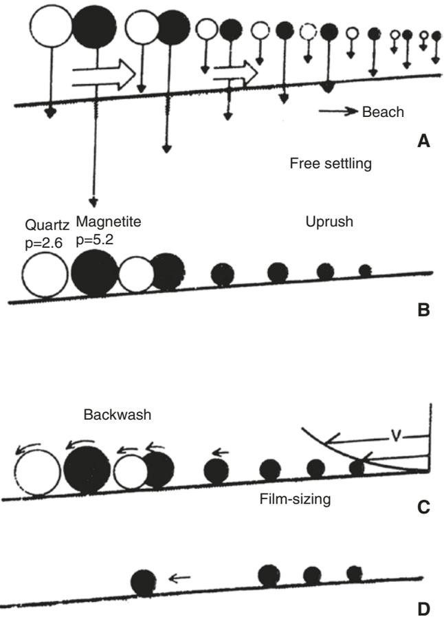
**Fig. 14.9** Origin of heavy mineral placers, schematic. (a) Suspended sediment particles are washed onshore with incoming waves, large and heavy ones first (black). (b) Resulting grain association is enriched in grains that settle easily. (c) Backwash rolls away large grains preferentially, owing to increase of water velocity off but still close to the floor (note  $v$  in inset). (d) Resulting well-sorted and heavy mineral assemblage (E.S., 1970. *Chem. Ing. Tech.* 42: A 2081)
