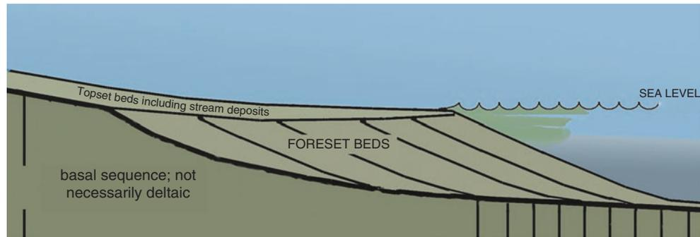
**Fig. 6.7** Schematic structural profile of a delta deposit, showing positions of topset, foreset, and bottom-set units (After a graph of US NEL geologist R. Dietz, as reproduced in A. Lombard, 1956. *Géologie Sédimentaire*, Vaillant- Carmanne, Liège. Modified and with color here added)
