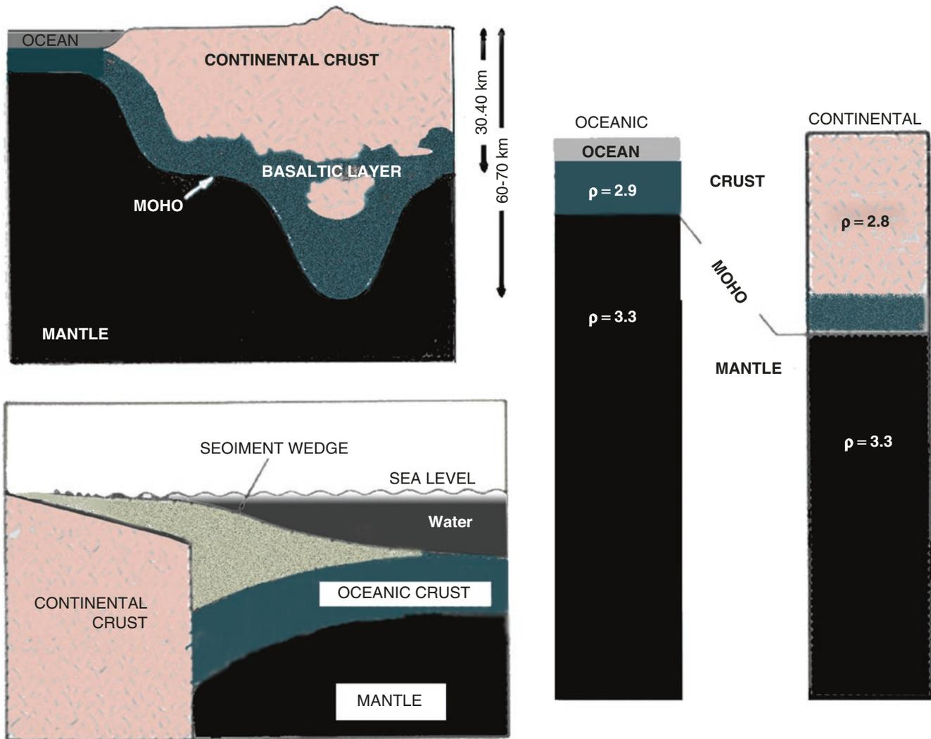
**Fig. 3.1** Schematic isostatic block models for the continent-ocean transition and the significance of the “Moho” as a crust-mantle boundary (Mainly after S. Uyeda, 1978)
