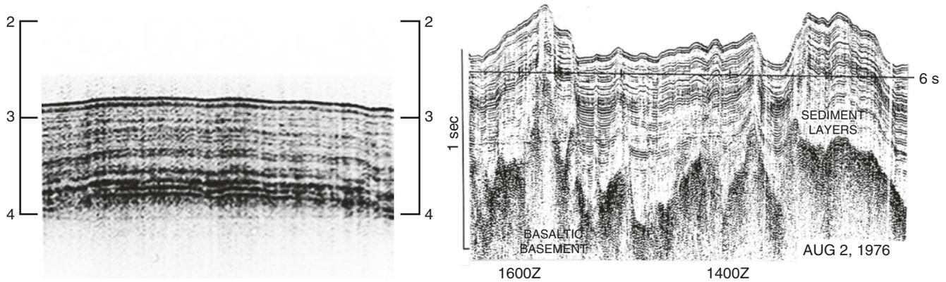
**Fig. 10.7** Evidence from seismic echo surveys that deep-sea sediments are surprisingly thin. Thickness scale: echo return time (sound velocity in sediment, 1500–2000 m per s). *Left*: shallow part of Ontong Java Plateau (ca. 100 million years; thickness in excess of 1 km in places);
