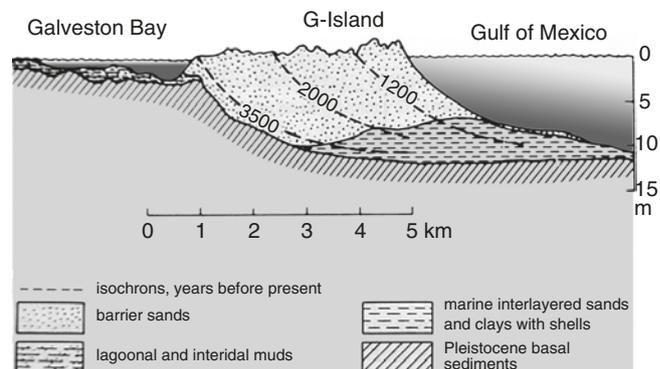
**Fig. 6.9** Structure of Galveston Island. Regressive sequence below the barrier beach near Galveston, due to high supply of sediment. Age: late Holocene (From J. R. Curran, 1969. In: D.J. Stanley (ed.) *The new concept of continental margin sedimentation*. Am. Geol. Inst., Washington, D.C. Shading here added)
