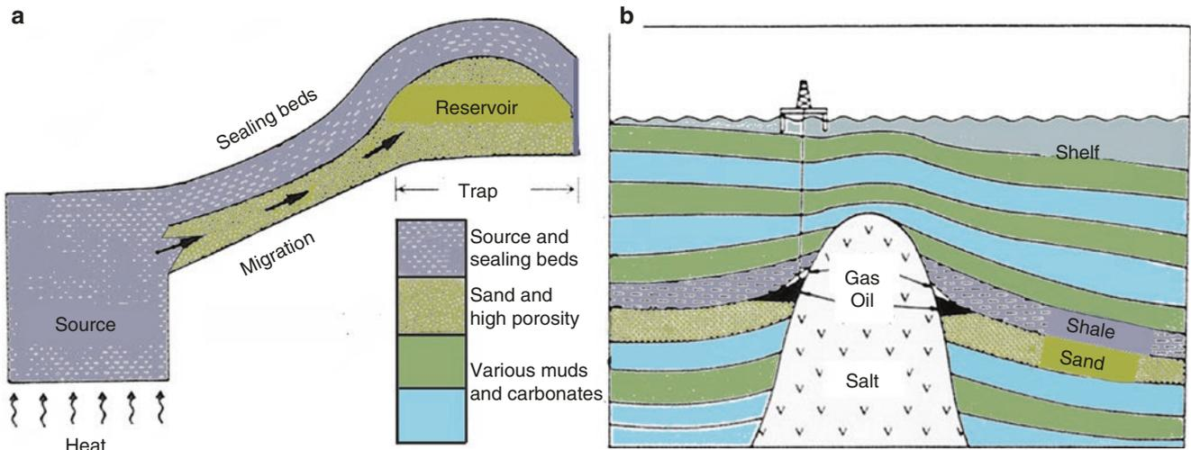
**Fig. 14.3** Schematics on hydrocarbon accumulation. (a) Basic elements of a petroleum reservoir system, with migration from heated source rocks to a porous reservoir. (b) Offshore salt dome tectonics generating trapping conditions
