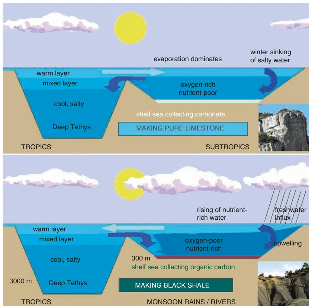
**Fig. 2** Eugen Seibold's scheme of making carbonate or organic-rich shale in shelf seas, depending upon the contrast in circulation in arid and humid regions. Upper panel (a): arid conditions, schematic; compare Persian Gulf. Lower panel (b): humid conditions, schematic; compare Baltic Sea. Inset photos: Mesozoic shelf deposits, marine carbonate rocks (arid) and black shale (humid) in southeastern France (for oceanography, see Sect. 9.5) (After ideas of E. Seibold, published in 1971)
