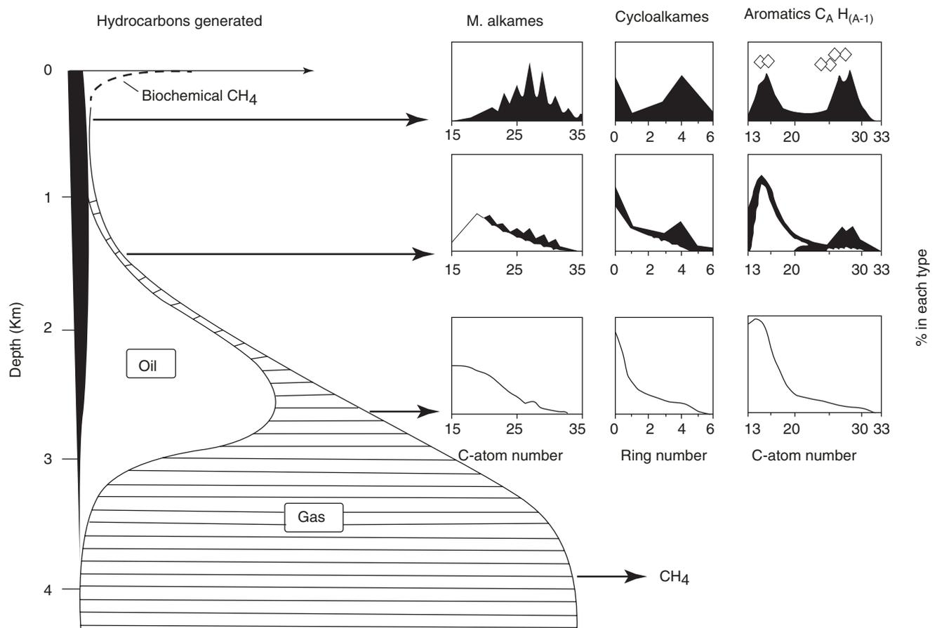
**Fig. 14.2** Origin of petroleum. After burial of the source material (black), carbon chains and rings are produced. Gas is produced under a large overburden and can help push the oil out during production (After
