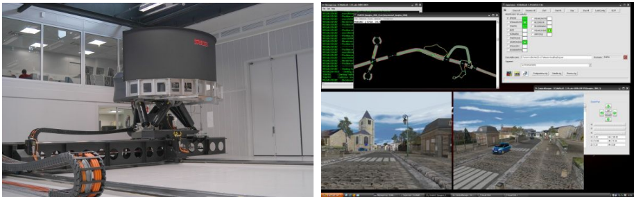
Fig. 5. The dynamic simulator Ultimate at Renault ( left ), and a screenshot of the SCANer TM software with two visuals outputs, the traffic and the supervisory modules ( right )
