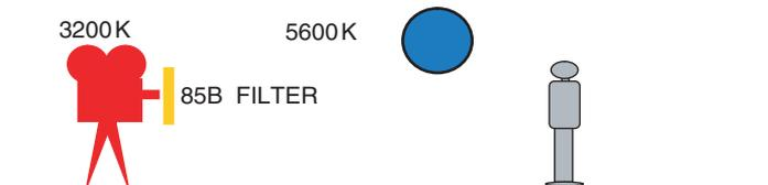
Here, an actor stands outdoors in 5,600K sunlight. There is 3,200K film in the camera. Shooting under these conditions will make the color on film too blue. Since the sunlight is too blue, a filter can be used to remove some of that blue light. On the subtractive color wheel, yellow is opposite blue (complementary color). Placing an orange-shish-yellow filter (commonly called an 85B filter) over the camera lens will absorb a portion of its complementary color (the
