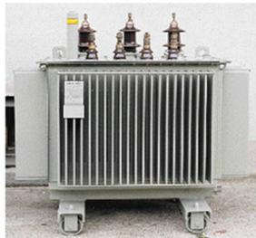
Distribution transformers receive electricity from the medium voltage network (e.g. 20 kV or 10 kV) and transform it to 380/230 V for distribution to the residential and small scale consumers. They are generally installed in prefabricated concrete containers in the streets.
