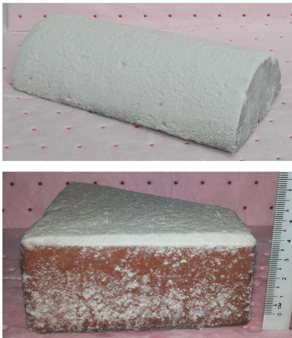
**Figure 2.4** Concrete and brick bio-coated with calcite.
