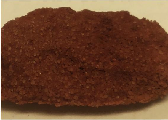
**Figure 3.4** Sand after bioclogging with iron-based biogROUT.
