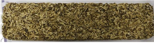
**Figure 16.5** Composite chitosan/sunflower stalk used for designing thermal insulation panels for existing buildings.
