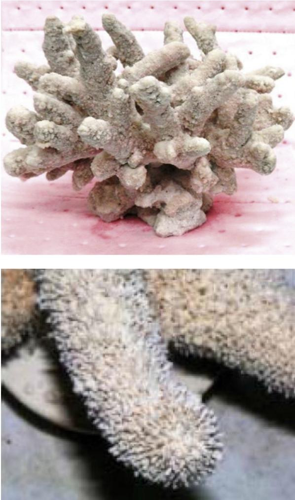
**Figure 2.5** Artificial corals biocoated with calcium carbonate minerals.
