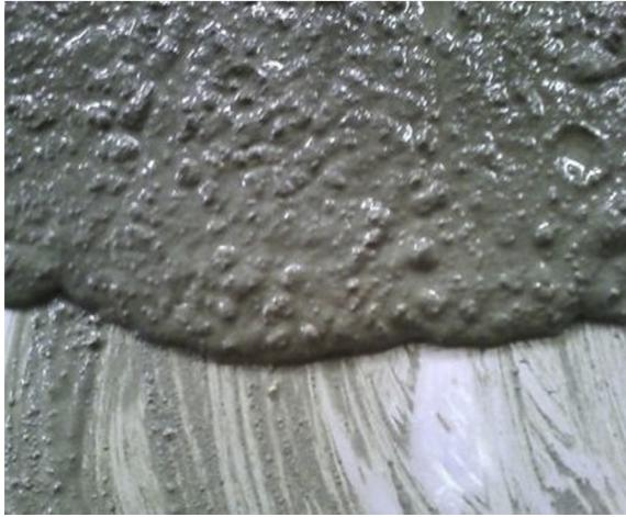
**Figure 8.6** Details of the edge of slump flow, SCC made with bioplasticizer. [Fernando Martirena et al. \(2014\)](#).
