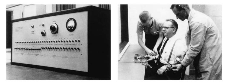
**FIGURE 2** This fearsome-looking "shock generator" led participants to believe they were administering electric shocks to another person, who was connected to the generator by electrodes that were attached to the skin. (Source: Copyright 1965 by Stanley Milgram. From the film *Obedience*, distributed by the New York University Film Library and Pennsylvania State University, PCR.)
