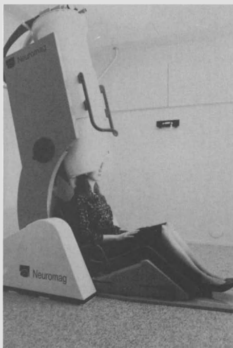
Fig. 1. Whole-scalp Neuromag-122™ neuromagnetometer. The measurements are performed in a magnetically shielded room
