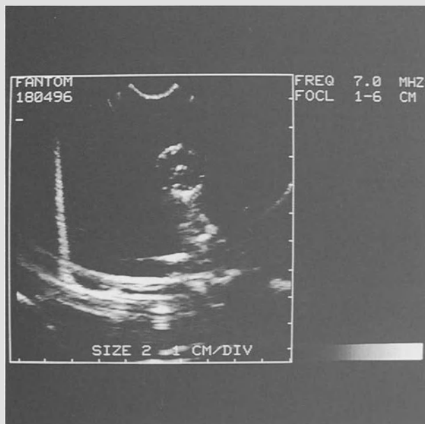
Fig. 2. MR and ultrasonic images of a gelatin phantom. The phantom consisted of a plastic rectangular box filled with hardened gelatine. Hollow tubes (10 mm diameter) containing vitamin capsules were imbedded in the gelatin in various planes. The phantom was scanned in the axial plane and registered in the OTS via 4 surface fiducials. (a) Shows the reformatted MR images in all three planes corresponding to the "virtual tip" in the ultrasonic beam as indicated by the cross hairs. (b) Shows the axial ultrasonic image of the target at this level. The tube wall and the MR target are clearly identified from the reflection artifacts
