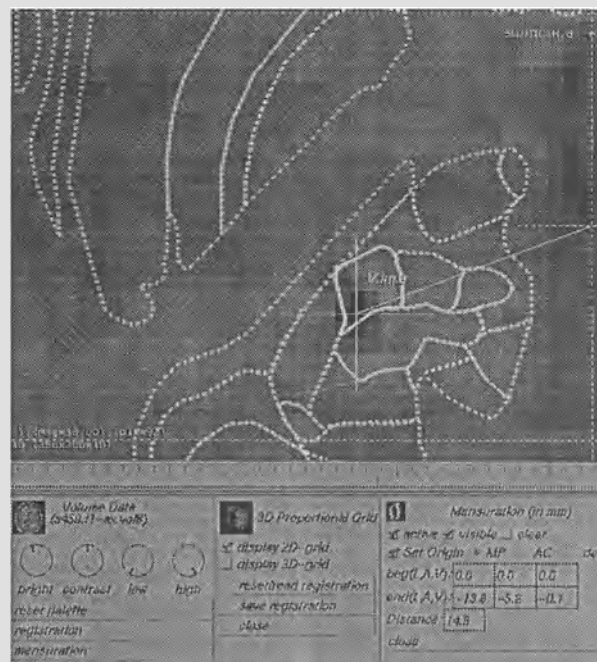
Fig. 5. Postoperative mensuration of the location of an electrode implanted in the right thalamus. Top: MRI image with the superimposed contours (the Vim.e nucleus is highlighted and labelled) and Talairach grids are highly magnified, and the target (marked by the cross) is measured with subpixel accuracy. Bottom-right: mensuration control panel segment. The intercommissural midpoint (MP) is set as the origin. The distance to the target, and the target lateral, anterior and ventral (L, A, V) coordinates are displayed
