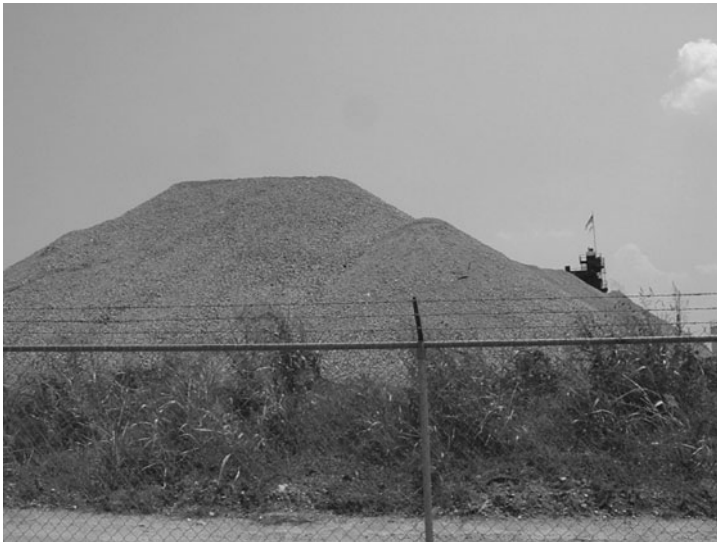
FIGURE 5.2.1 Stockpile of crushed concrete at the Sloan Construction asphalt plant in Columbia, S.C., ready for reuse. The concrete comes from the demolition of dormitories at the University of South Carolina, only a few miles away. (Photograph taken August 2007.)
