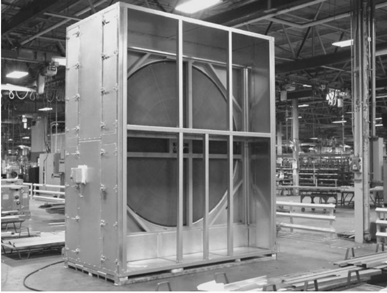
FIGURE 6.7.1 Trane CDQ (Cool, Dry, Quiet) is a desiccant wheel which is placed in series with the cooling coil and can help provide dry air to a space for better humidity control. (Photograph Courtesy Trane.)
