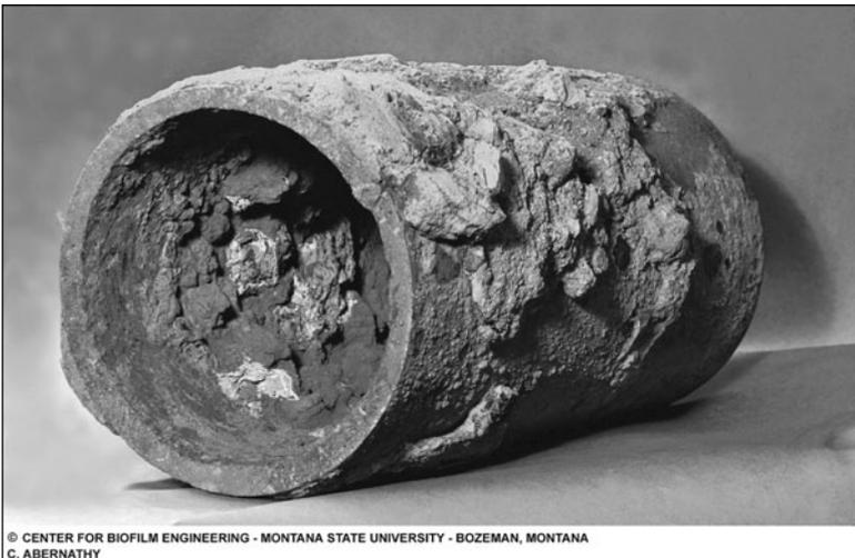
Figure 4.2 Biofilm corrosion. This pipe has been almost completely occluded by biofilm, which has dried and hardened. Few technologies exist for removing biofilm from living or nonliving surfaces. (Courtesy of Center for Biofilm Engineering, Montana State University)
