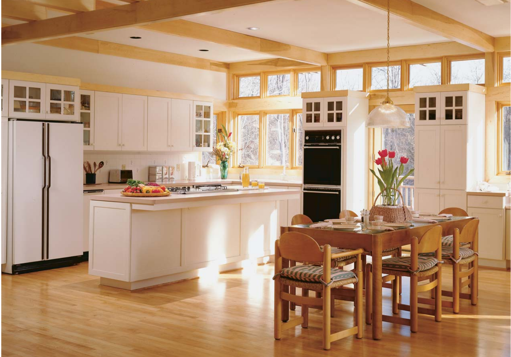
Increasing the ceiling height in this kitchen and dining area from 8 ft. to 9 ft. led to the inclusion of transom windows above the door and main windows. A change in stud length often has such ramifications throughout the house, which can add substantially to the cost.
