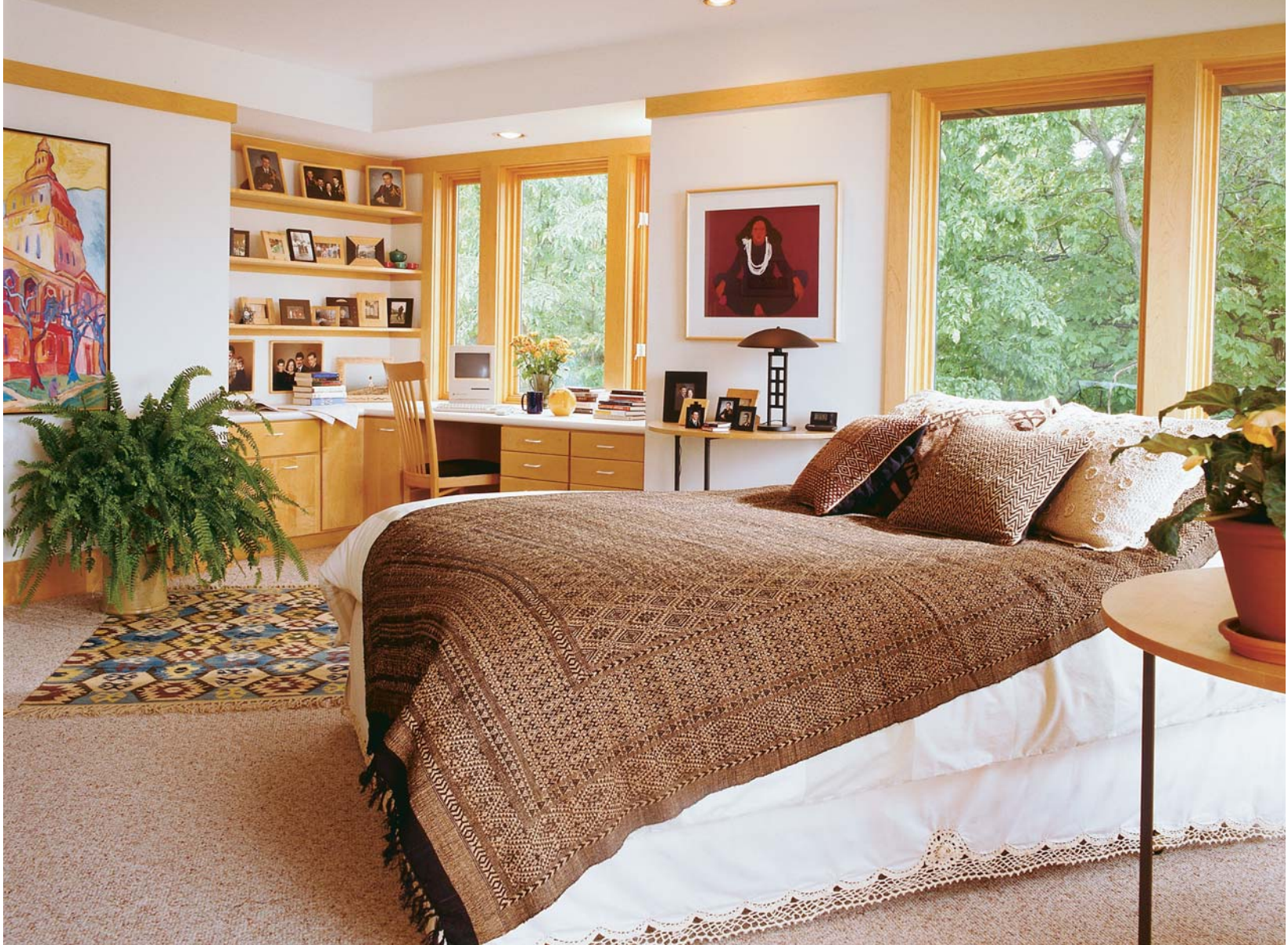
An alcove in the master bedroom serves as an office area. The alcove is created by a lowered ceiling and a window bay that extends to two stories—on the first floor it accommodates a kitchen bay (see the photo on p. 111).
