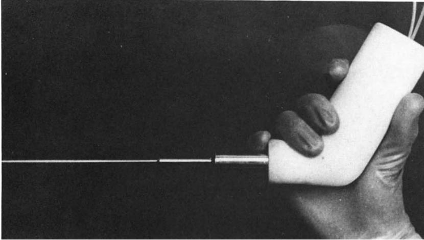
**Figure 2.** Device for cryosurgery, of the author's own construction.
