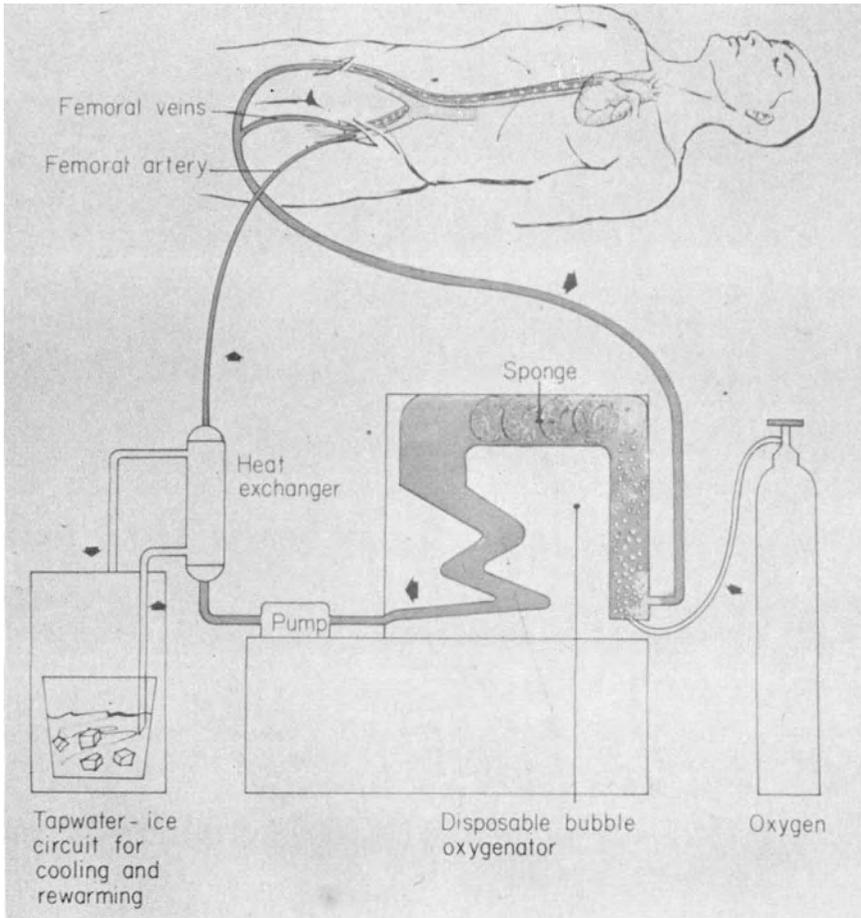
**Figure 3.** The extracorporeal circuit for deep hypothermia.
