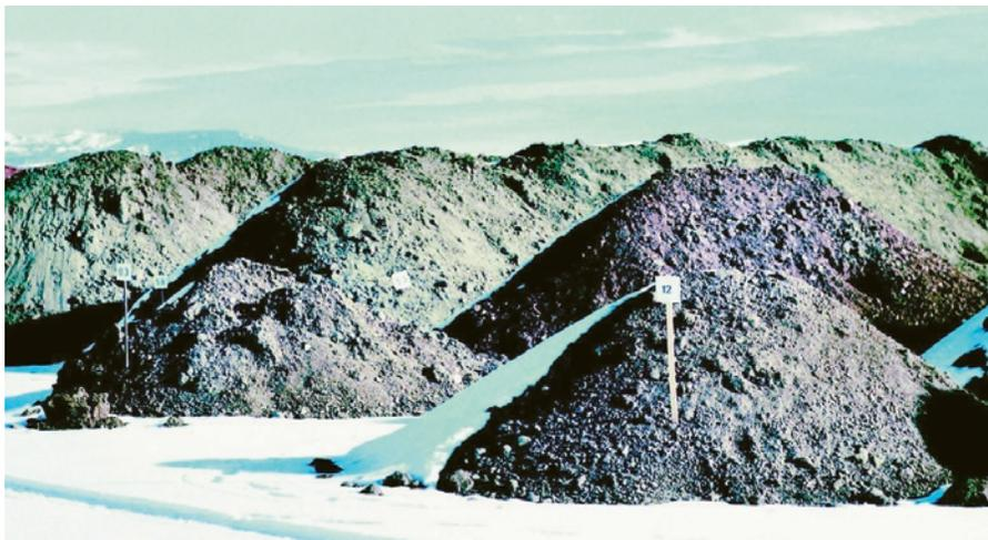
This petroleum-contaminated dirt was mixed with clean dirt and manure before being injected with microbes. The microbes fed on the petroleum's hydrocarbons, converting the harmful materials into carbon dioxide and oxygen.
