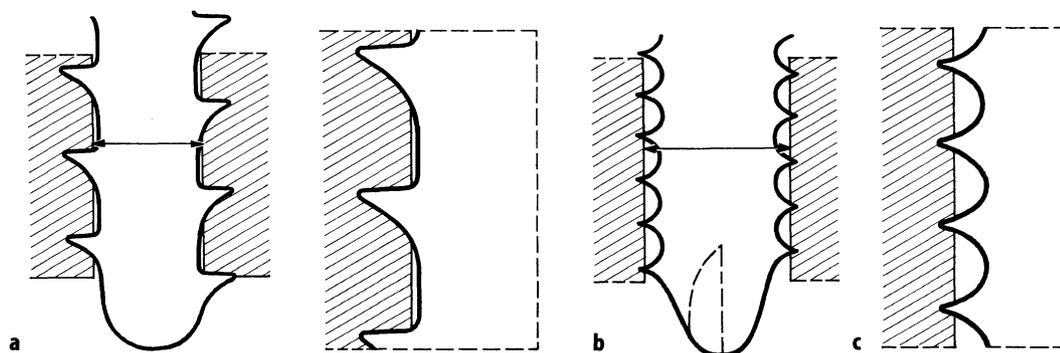
**Fig. 2.1a–c.** Non-self-tapping screw (a) and self-tapping screw (b). The pilot hole for the self-tapping screw has to be larger, and the screw threads do not penetrate as deeply into the bone (c)
