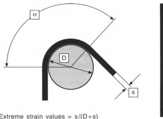
**Fig. 3.5.** Strain values on the surface of a plate in the case of contouring (bending to a curvature of diameter  $D$ ). Extreme strain values =  $s/(D+s)$
