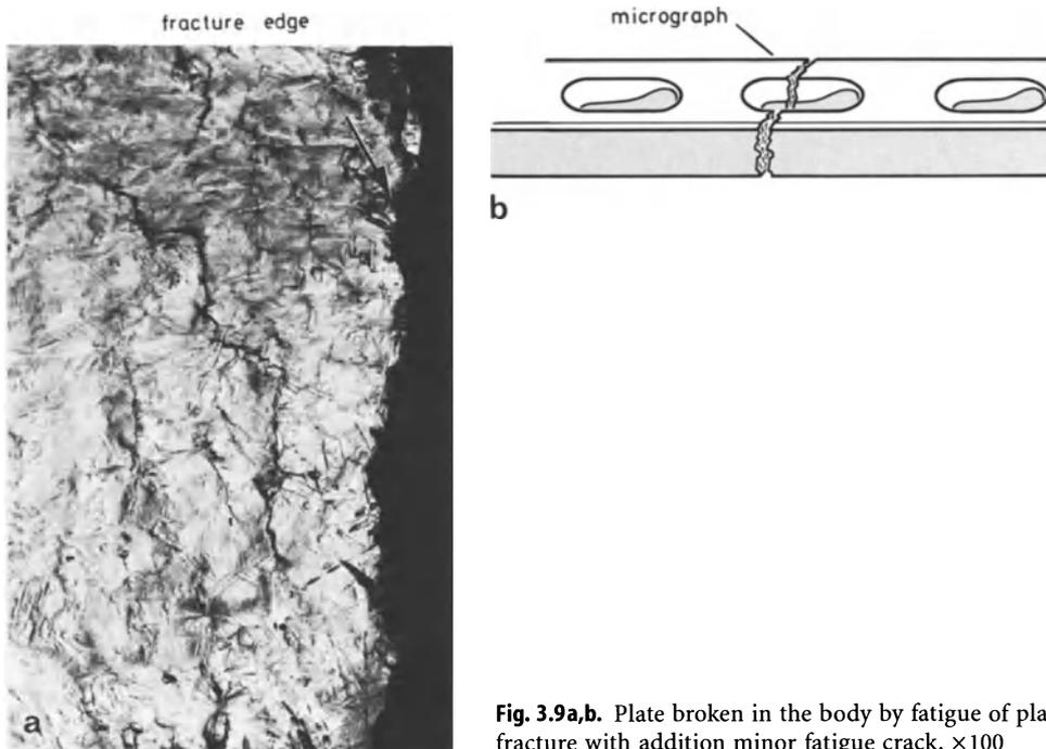
**Fig. 3.9a,b.** Plate broken in the body by fatigue of plate surface adjacent to fracture with addition minor fatigue crack.  $\times 100$
