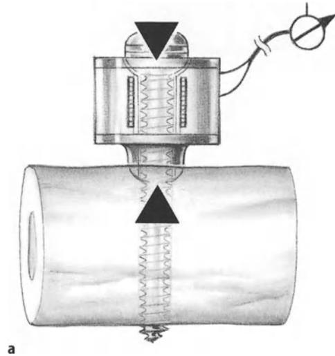
**Fig. 1.31a,b.** Measurement of screw compression in vivo (Blümlein et al. 1977). **a** Instrumented washer for in vivo measurement of screw compression. A washer is fitted with strain gauges and a transcutaneous wire connection. **b** Recording compression exerted by screws in vivo. Three different groups of initial compression and their changes in vivo are plotted. Over a period of 16 weeks, the compression regressed very slowly
