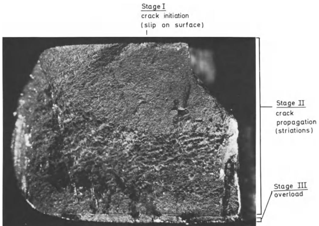
**Fig. 3.10.** Macroscopic view of fatigue fracture surface of a broken plate. The three main stages of fatigue are indicated
