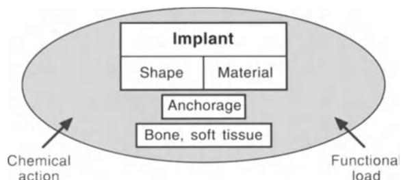
**Fig. 3.1.** Interaction between implant and environment (biomechanical structure)
