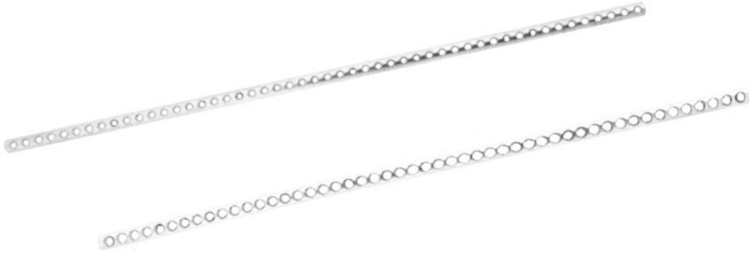
**Fig. 2.46.** Cuttable plates are made in two sizes: the 1.5 and 2.0-mm plates possess 50 round holes and have dimensions of 1.0×7×300 mm. The plates may be stacked on top of one another, either with a plate of the same size or with a smaller
