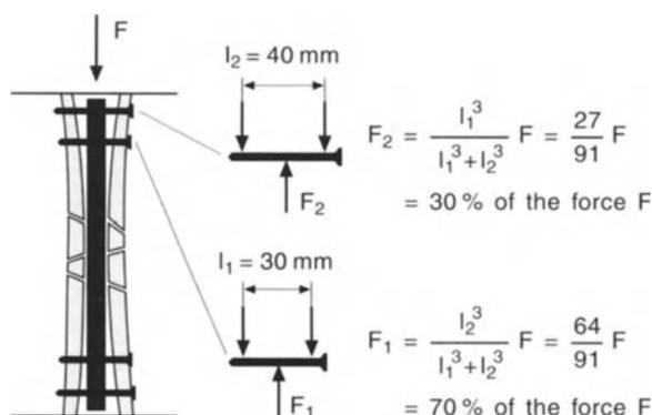
Fig. 3.3. Load distribution for locking bolts: an example
