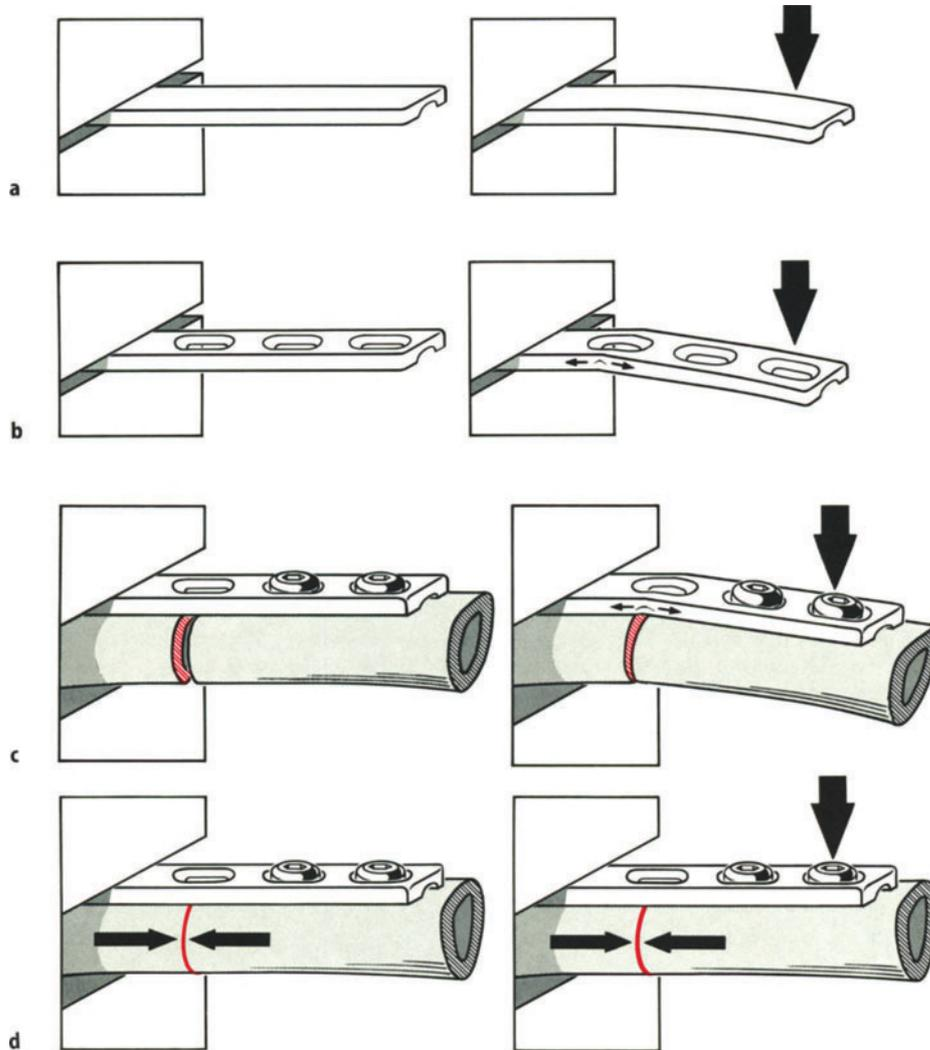
**Fig. 3.14a–d.** Stress concentration in plate holes. **a** If a plate without holes is bent, stresses are distributed evenly over the plate. **b** If the plate contains a hole, stresses concentrate there, at the smallest cross-section. **c** If, at the same time, the plate is supported, e.g., by a bone, the bending effect on the plate is reduced. However, when support is lacking underneath the plate hole because of a persistent fracture gap, the stresses at
