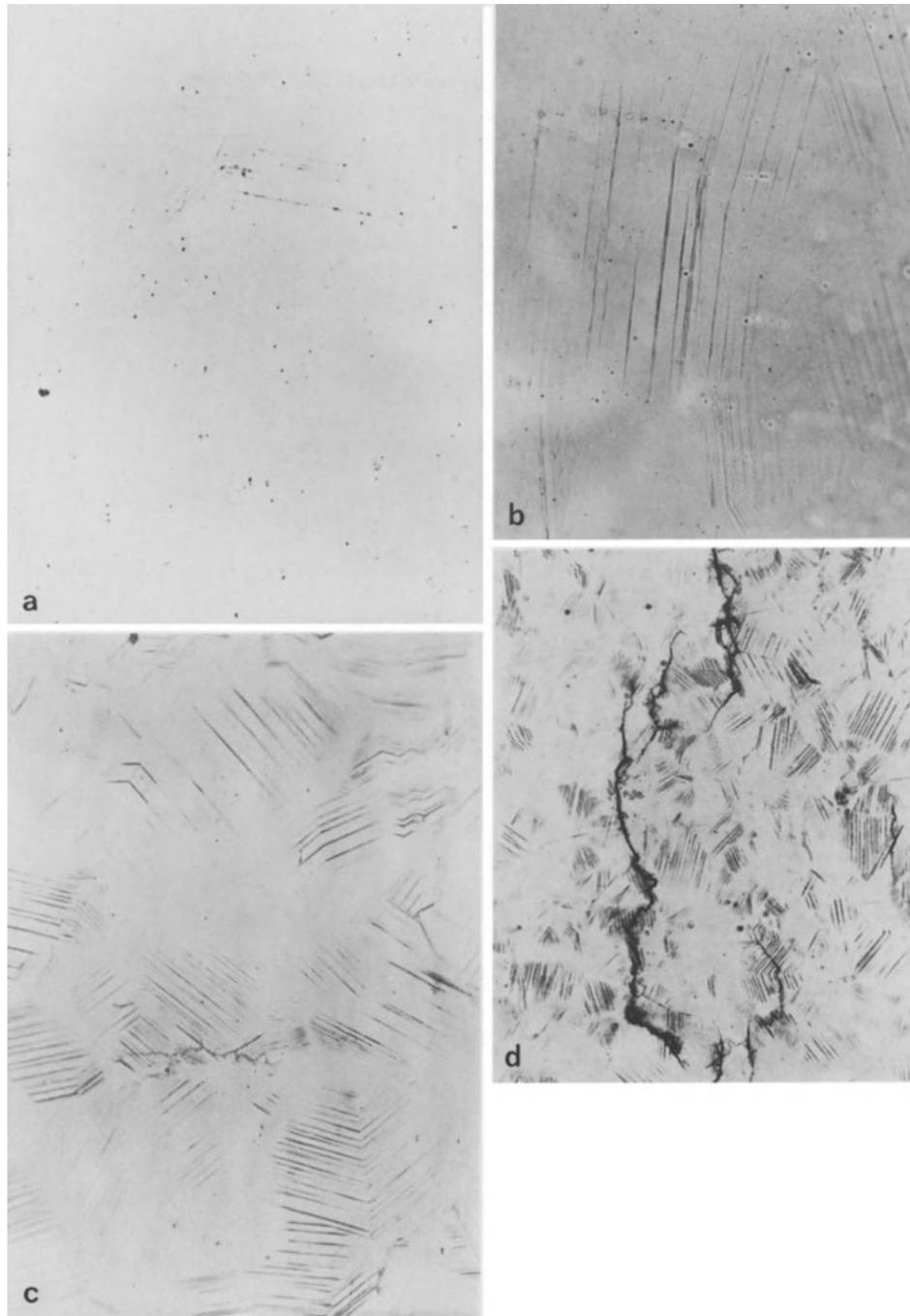
**Fig. 3.7a–d.** Development of fatigue cracks on stainless steel implant material during in vitro testing in Ringer's solution. (The micrographs show the implant surface after a certain number of load cycles.) **a** After 500 cycles: single slip systems
