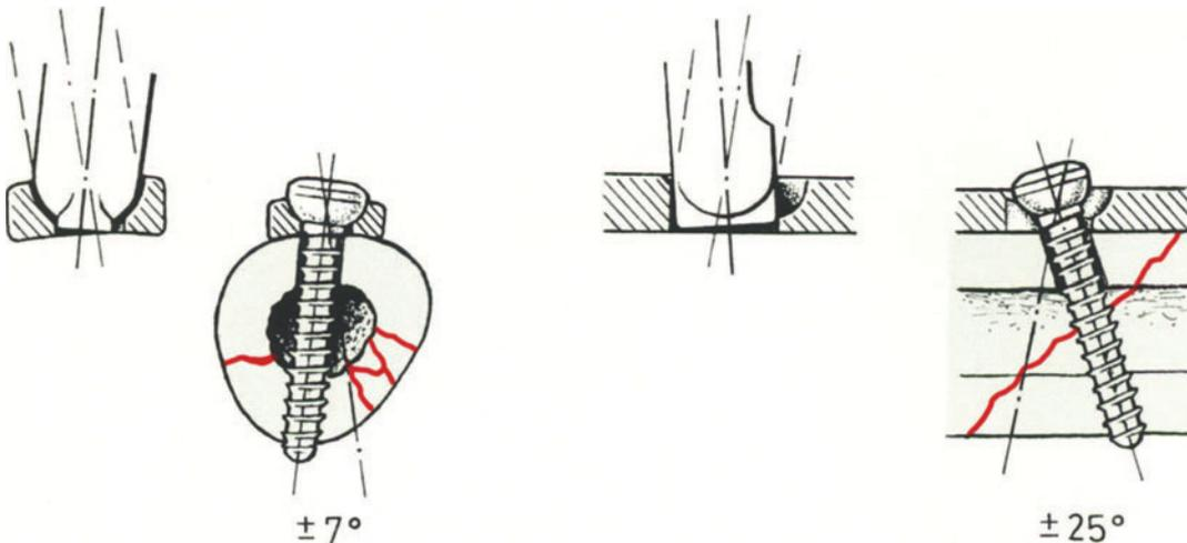
**Fig. 2.20.** The interplay between the spherical screw head and the geometry of the screw hold permits the angulation of the screws in all directions (maximum 25° longitudinally, 7° sideways)
