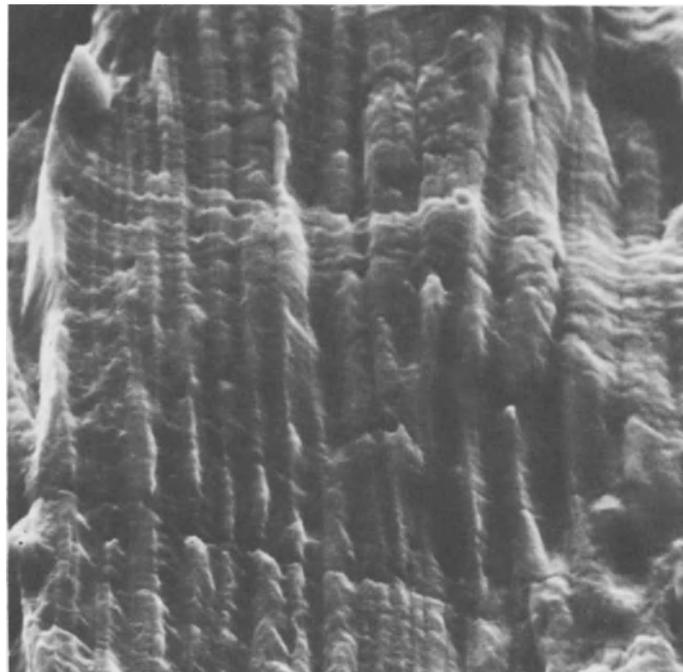
**Fig. 3.11.** SEM micrograph. Fine parallel horizontal lines show typical fatigue striations caused by single load cycles (propagation stage of Fig. 3.9).
