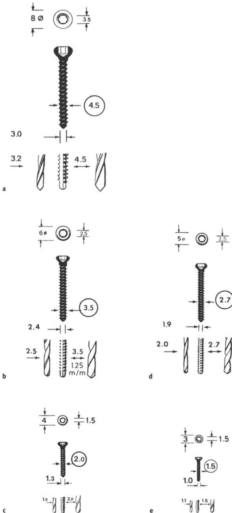
**Fig. 2.2a–e.** Cortex screws. **a**
