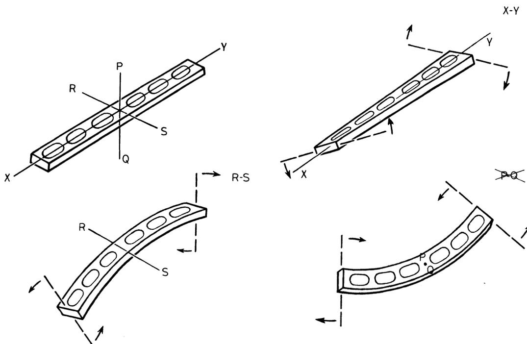
**Fig. 2.30.** A narrow or a broad dynamic compression plate (DCP) can be twisted about its  $X$ - $Y$  axis and bent about its  $R$ - $S$  axis. It resists strongly any attempt to bend it about its  $P$ - $Q$  axis
