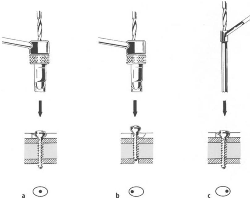
**Fig. 2.19a-c.** The drill guides for the dynamic compression plate (DCP). **a** Neutral drill guide (green; color not shown here). It places a screw 0.1 mm from the end of the slope, inducing some axial compression. **b** Load drill guide (yellow; color not shown here). It places a screw 1 mm from the end of the slope. **c** The hole for buttress function, drilled using the double drill sleeve
