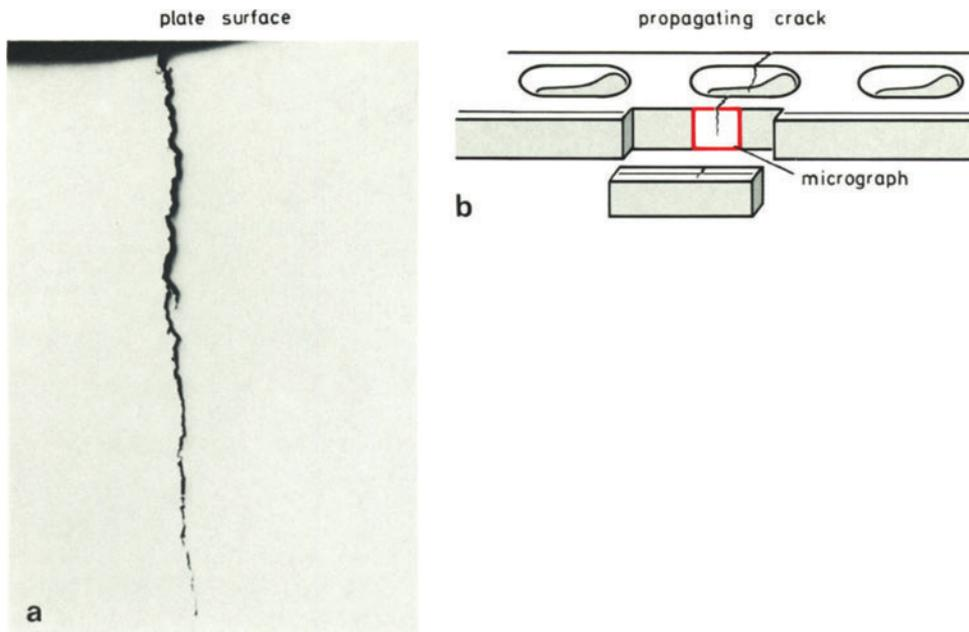
**Fig. 3.8a,b.** Fatigue crack propagation through plate shown on longitudinal section through plate.  $\times 110$
