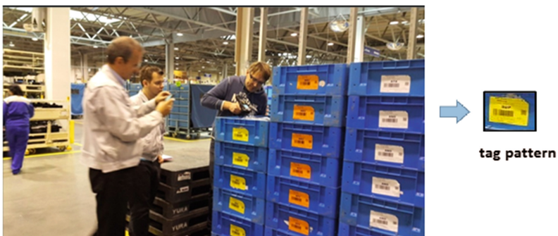
Fig. 1. Special RFID tag, which can easily recognized by computer vision system.
