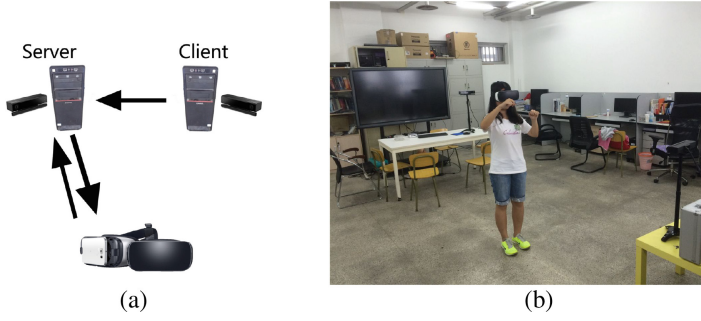
Fig. 1. The proposed wireless Kinect sensor network system. (a) The framework of the multiple Kinect sensors integration. (b) A scene of the VR application using the proposed system with two Kinect sensors.
