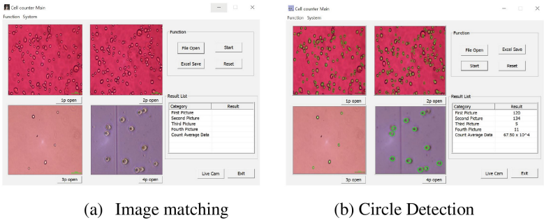
Fig. 5. An example of the developed cell counting program (Success). (a) Image matching (b) Circle Detection
