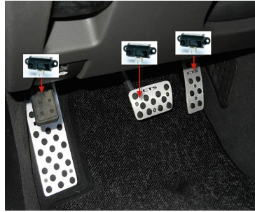
Fig. 5. Installation of distance measurement module sensor [5]
