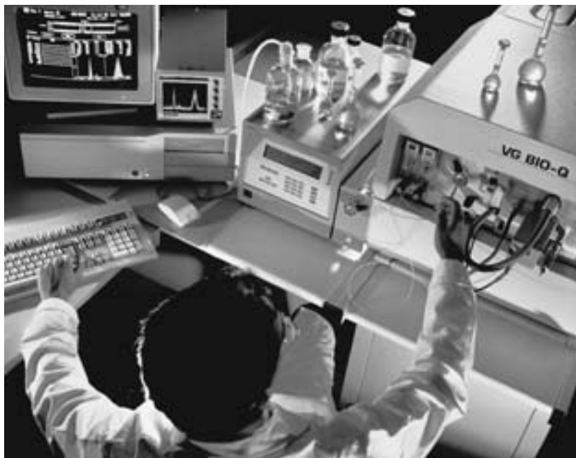
A scientist inserts a sample to be tested into the mass spectrometer shown here. (G. Tompkinson/Photo Researchers, Inc.)
