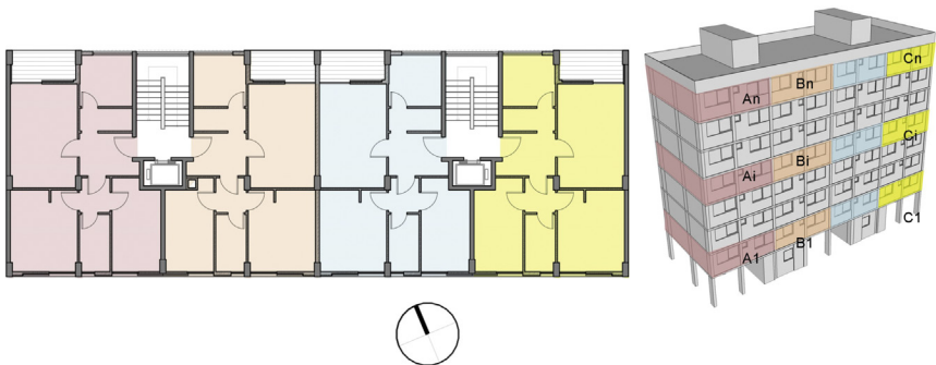
Figure 2.45 Apartments as thermal zones in the selected building block (T7) in Peristeri.
