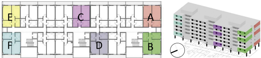
Figure 2.44 Apartments as thermal zones in the double block building (B6) in Peristeri.
