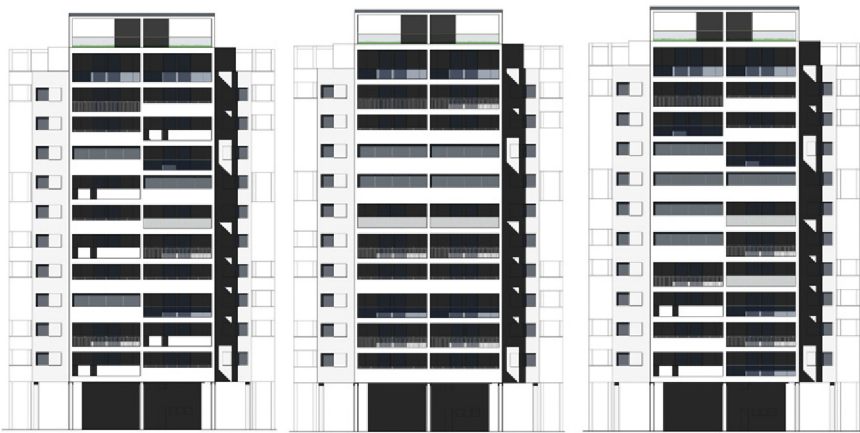
Figure 3.13 Combination of additions on the top (new residential units) and on the elevation of the buildings with new façade solutions selected from the abacus for the west façades in the tower building type.
