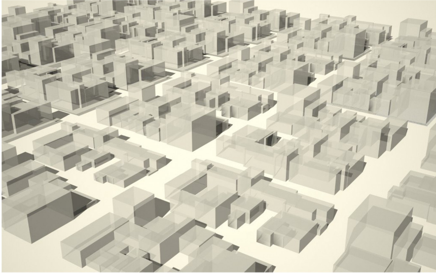
Figure 2.10 An example of the 3D models used to calculate Ae/V ratio for different urban block types in the homogeneous districts.
