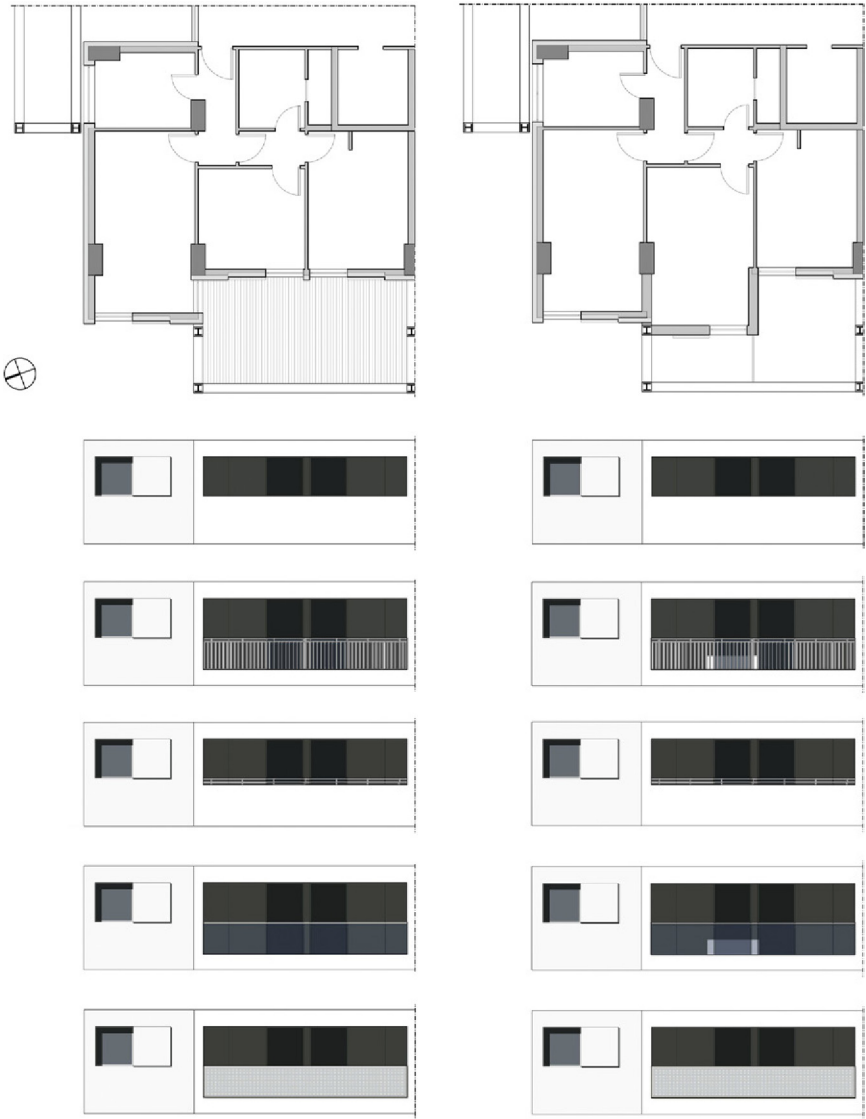
Figure 3.11 Abacus of modular options as a function of possible energy retrofitting scenarios and users' requirements in the west and east orientation of tower building type in Peristeri. (Facade insulation, window replacement combined with additional space for balconies, on the left, or additional space both for the room and for the balcony, on the right).
