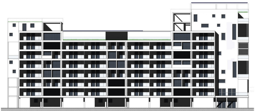
Figure 3.15 Designed scenarios on the west façade of the double building block B6. New residential units both on the south and north side of the block building are combined with add-ons and new façade solutions in the existing residential units.
