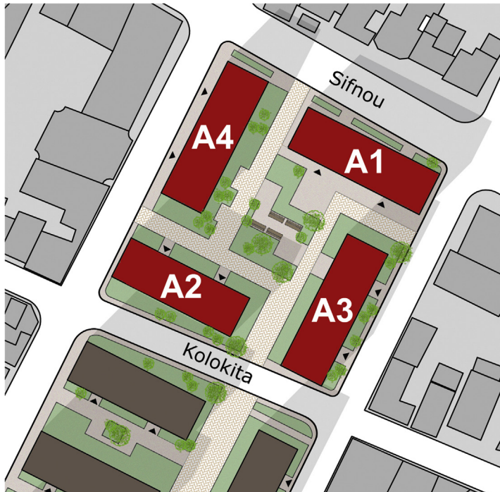
Figure 2.33 Type A buildings in the Aghia Varvara urban compound. Different subtypes (A1, A2, A3, A4) are identified as a function of different exposures in relation to the sleeping and living areas of the single residential units.
