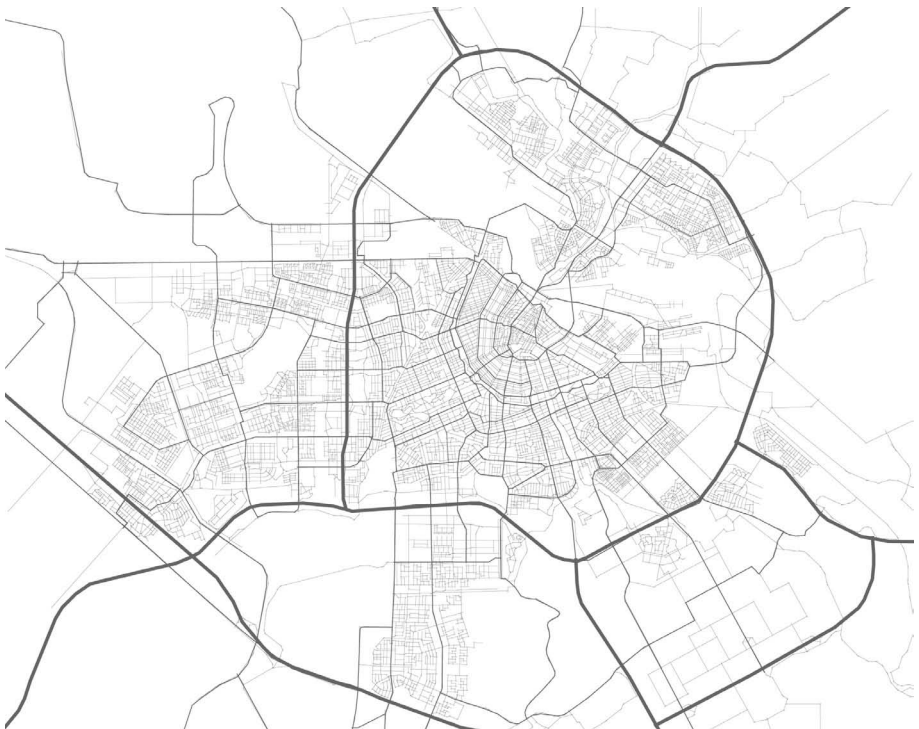
Figure 1. The breakdown of place- region strata in Amsterdam (Bruyns & Read, 2007); metropolitan network (dark lines, bold), middle-scale network (dark grey), and local network (light grey)
