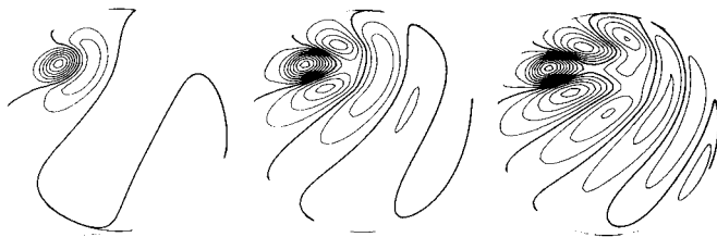
Fig. 10.15 The vorticity pattern generated on a sphere when a constant angular velocity westerly flow impinges on a circular forcing centered at 30^\circ\text{N} and 45^\circ\text{W} of the central point. Left to right, the response at 2, 4, and 6 days after switch on of the forcing. Five contour intervals correspond to the maximum vorticity response that would occur in 1 day if there were no wave propagation. Heavy lines correspond to zero contours. The pattern is drawn on a projection in which the sphere is viewed from infinity. (After Hoskins, 1983.)
