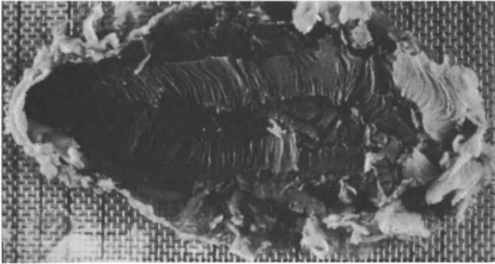
Figure 1.2. A laboratory simulation of lava flow emplacement using carbowax in a sugar water solution that reproduces the essential rheologic properties of flowing basalt. Lines on the floor are 2 cm apart; vent is to the left. Solid wax is light; liquid wax is dark. Courtesy of Jonathan H. Fink, Arizona State University, and Tracy K. P. Gregg, SUNY-Buffalo.
