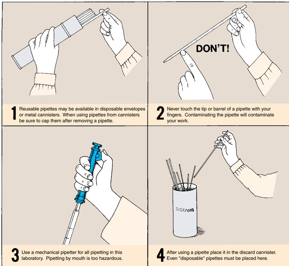
**Figure 23.2** Pipette-handling techniques
