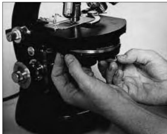
**Figure 3.6** Alignment of the annulus and phase ring on this Zeiss microscope is achieved by adjusting the two knobs as shown.
