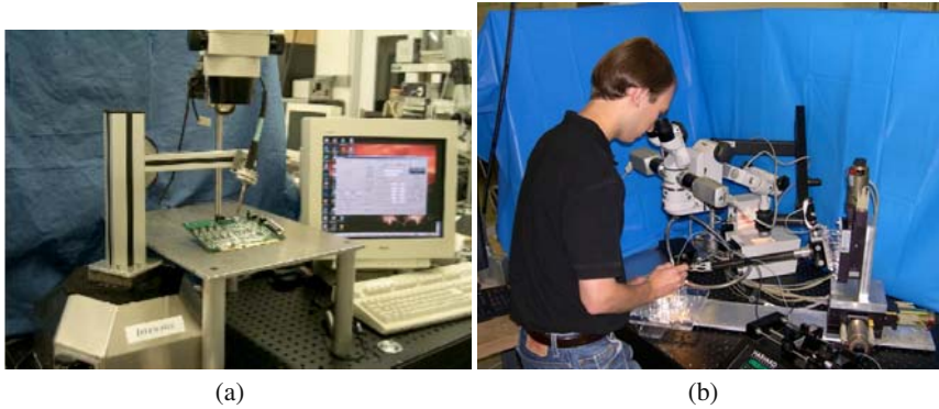
Fig. 4.3 Two applications of virtual fixture: (a) the InvenioSix high-precision robot in a configuration to support fine lead soldering; and (b) the latest generation SHR in a configuration designed for eye surgery
