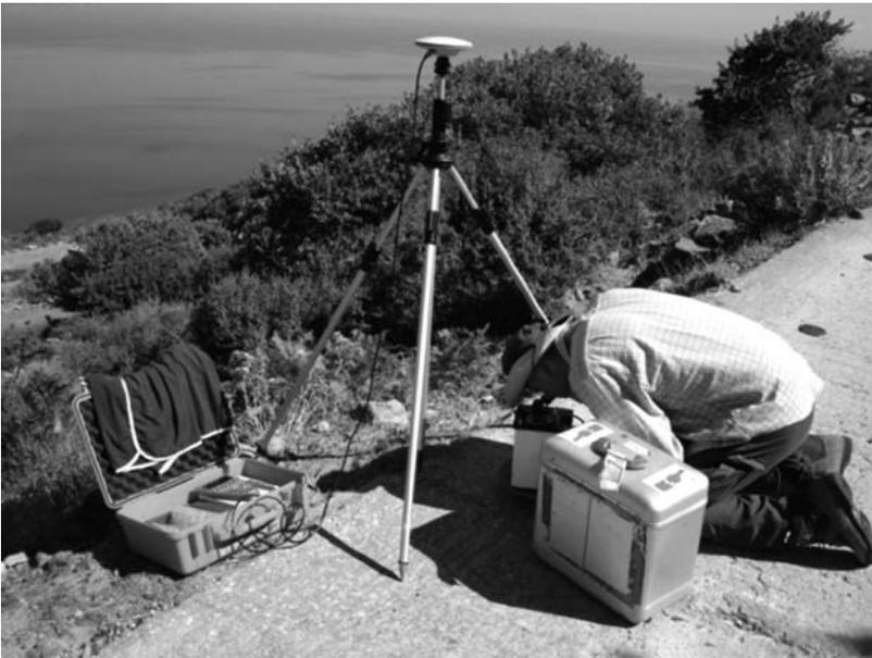
**Figure 1** A possible arrangement for the simultaneous occupation of a benchmark using a roving GPS receiver and a portable field gravimeter (photo credit: L. Wooller).
