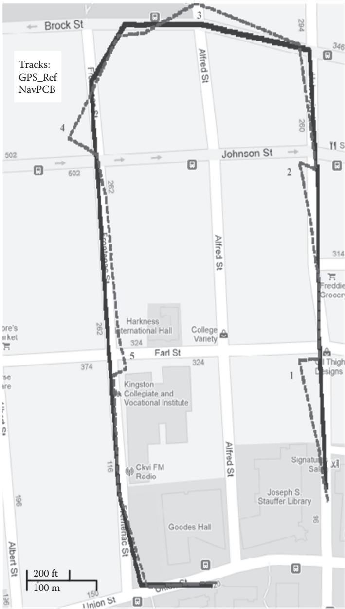
FIGURE 7.15 Field Test II (C): GPS trajectory vs. in-vehicle trajectory with five GPS outages.
