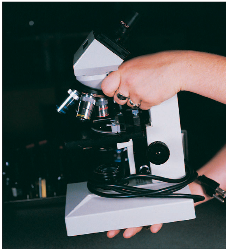
Figure 1.9 Method used to carry the light microscope.
