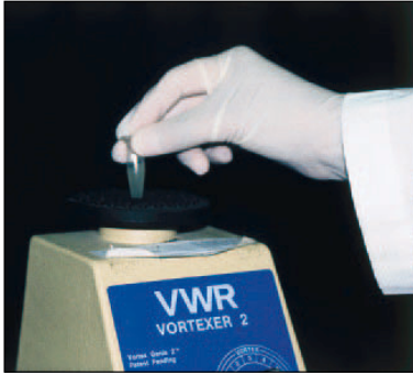
Figure 31.4 Vortex the sample for 2 minutes at the highest setting. This mechanically shears the DNA, generating fragments that are about 20 kilobases (kb). Later, you will further fragment the DNA with the restriction enzyme EcoRI.
