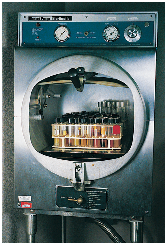
Figure 17.2 An autoclave, used to sterilize media.
