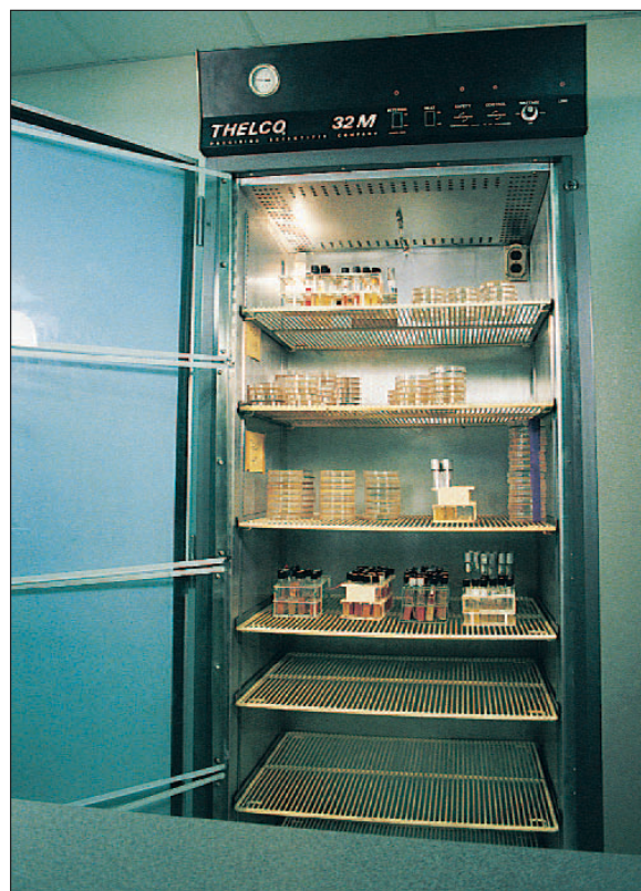
Figure 17.10 A laboratory incubator. A temperature of 35°C will encourage rapid bacterial growth.
