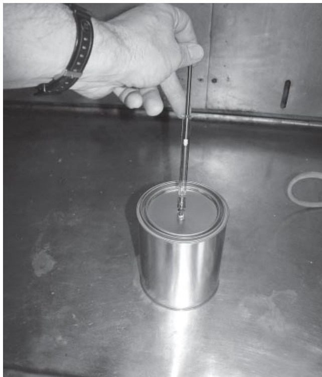
Figure 3.3 Using a gastight syringe to withdraw a sample of headspace from a fire debris sample. The headspace sample, about 500 \mu\text{L} , is injected directly into the GC–MS injection port.
