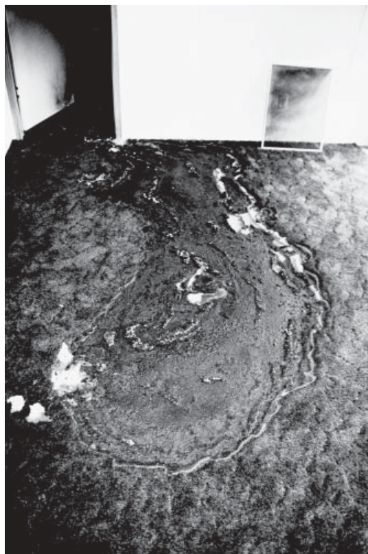
Figure 3.1 “Obvious pour pattern.” The only surface that was burned in this mobile home was the floor. There were no furnishings in the house. The carpet was tested and found to be positive for the presence of a medium petroleum distillate such as mineral spirits or charcoal lighter fluid. This is a unique case where visual observation alone can lead to valid conclusions about what caused the pattern. ( See insert for color representation. )
