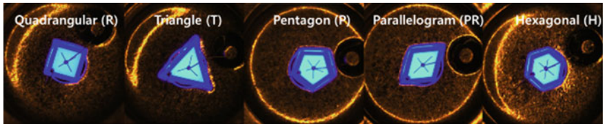
Fig. 12.4 Emission images of scribed polygonal LEDs with TO-can package at an injection current of 120 mA
