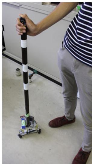
Although the conventional guide dog robots cannot climb of stairs, because of this light, this device can go up and down stairs along the railing by lifting. In addition, because it is small compared to the guide dog robots, this can run also in the room of the narrow passage.
