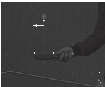
Fig. 9.8 Motion vectors for block matching estimation between frame #1 and frame #0 of the Table Tennis sequence
