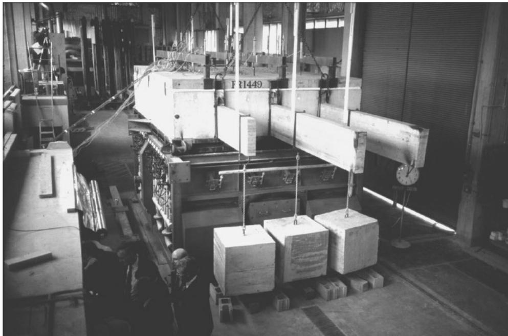
**Figure 9.19** Fire resistance test of glulam beams; the beams span a 4 m long furnace with loads applied using concrete blocks
