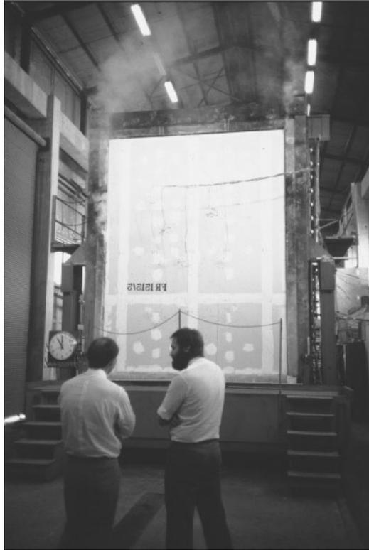
**Figure 10.7** Full-scale fire resistance test of a light timber frame wall
