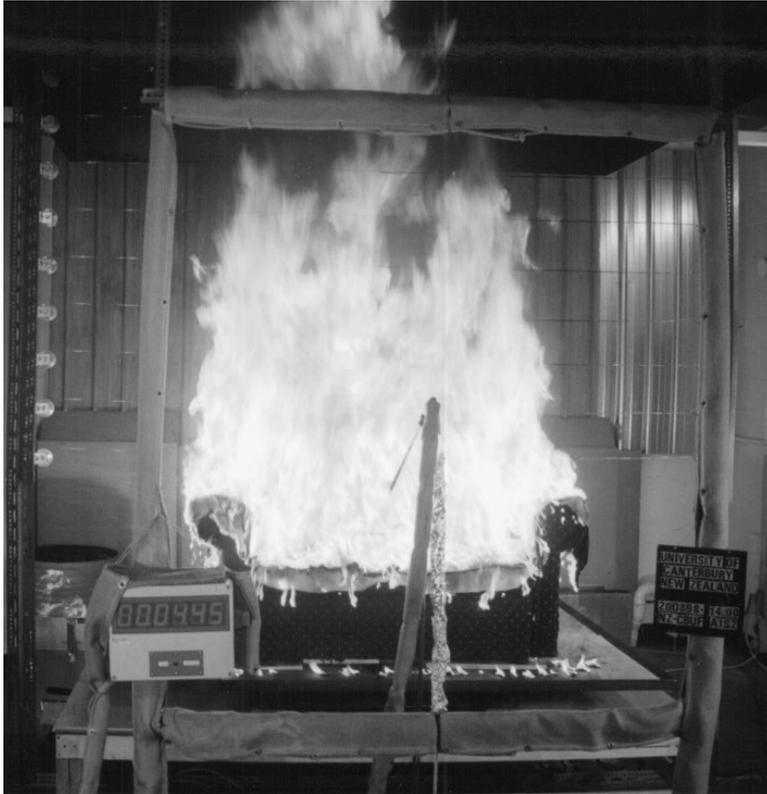
**Figure 3.1** A burning sofa in a furniture calorimeter test. If this sofa was burning in a room, the room would be full of toxic smoke
