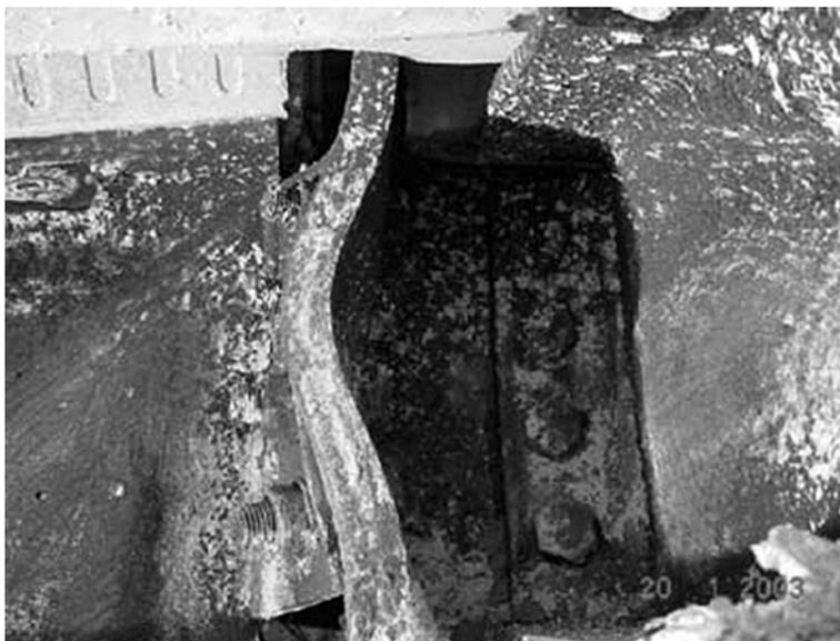
**Figure 11.12** Column flange buckling in Cardington Test 7. Reproduced from Wald *et al.*, 2006 with permission from Elsevier Science
