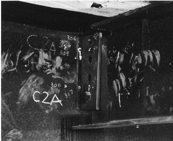
**Figure 11.11** Connection failure, during cooling, in Cardington tests. Courtesy of B.R. Kirby, Corus Fire Engineering
