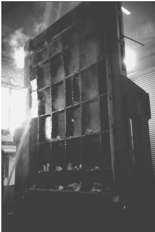
**Figure 10.12** Residual charred studs of a light timber frame wall after a full-scale fire resistance test
