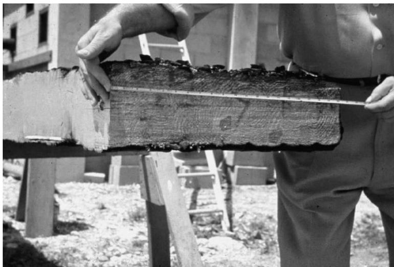
**Figure 9.20** Residual cross section of a large glulam beam after a fire test. Reproduced by permission of American Institute of Timber Construction
