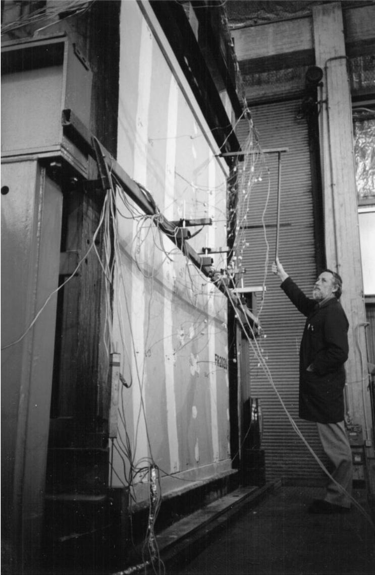
**Figure 10.16** Full-scale fire resistance test of a light steel frame wall. The wall has deflected inwards towards the furnace due to thermal bowing
