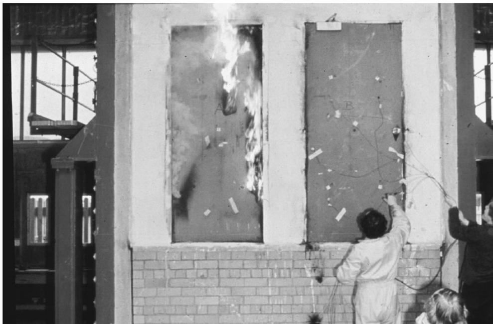
**Figure 4.12** Fire resistance test of two doors. The door on the left has had an integrity failure, as shown by penetration of flames and hot gases. Reproduced by permission of Building Research Association of New Zealand
