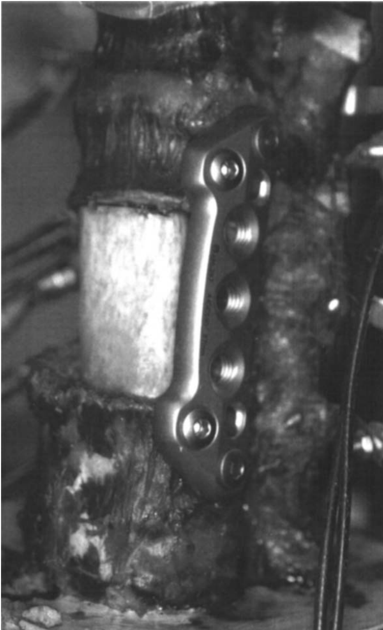
Figure 1 The ATLSP device with four constrained unicortical screws applied between T12 and L2. This constraint prevents angular rotation or backing out.
