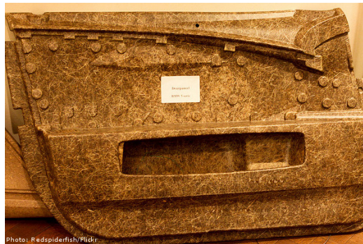
Figure 5.18 A BMW door panel made out of hemp. (source: TruthOnPot.com, 2013)
