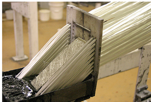
Figure 2.14 Open-bath pultrusion forming (source: Martin Pultrusion)
