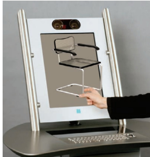
Figure 3. (a) stereoscopic glasses (HMD), (b) autostereoscopic 3D displays (Adapted from 3DTV- Display Techniques: A Survey, 2005)
