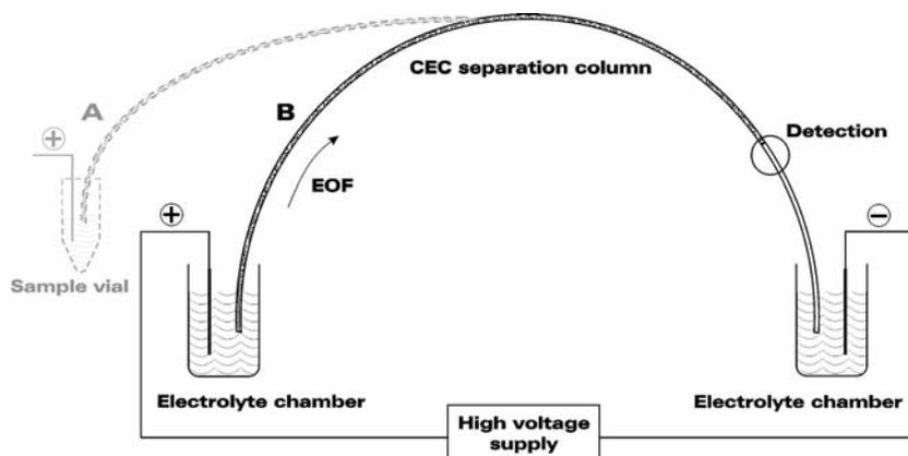
**Fig. 2** Schema of electrochromatograph. (A) Electrokinetic sample injection. (B) CEC separation.
