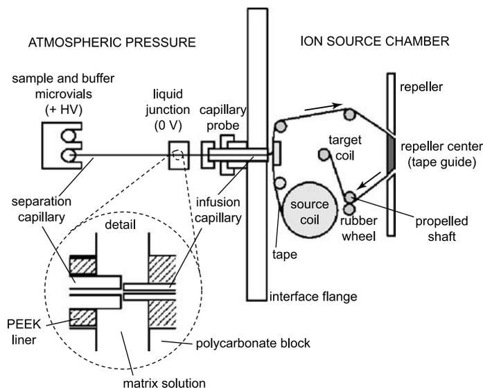
**Fig. 3** Schematic of the on-line coupling of CE to MALDI. (From Ref. [11].)
