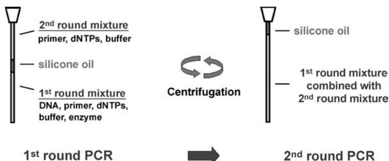
**Fig. 1** Schematic sketch of single-tube two-round real-time PCR in glass capillaries on the LightCycler instrument. (View this art in color at [www.dekker.com](http://www.dekker.com).)
