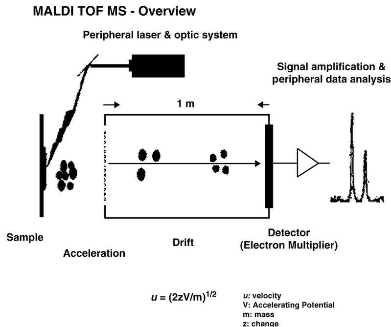
**Fig. 1** Depicted is a schematic overview of the MALDI-TOF process. The text provides a detailed description.
