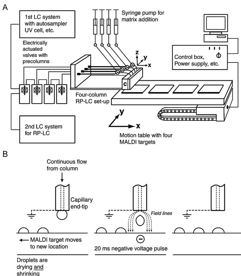
**Fig. 1** Automatic deposition of effluent from cLC directly down to a MALDI target plate. A) The automated off-line system for cLC-MALDI. B) Deposition of the effluent from the LC column down to the target plate by application of a negative voltage. (From Ref. [4].)
