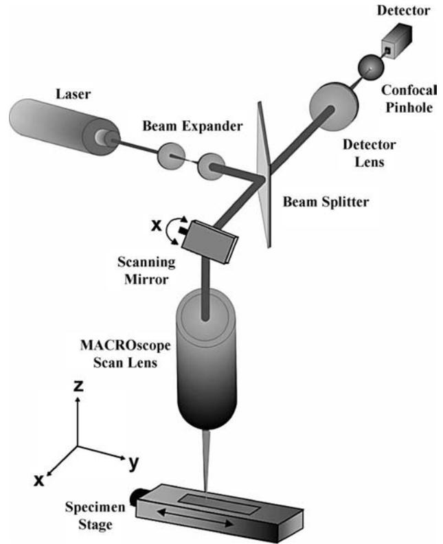
Fig. 3 Widefield confocal scanning laser MACROscope<sup>®</sup>.
