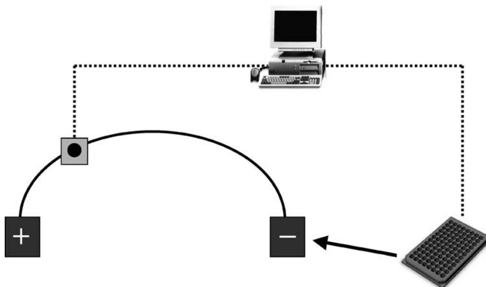
**Fig. 1** Simple representation of a CGE apparatus. The + and – represent the anode and cathode, respectively, joined through a capillary (solid line). The sample is loaded automatically and the end products are detected through a laser–CCD system (■). Software allows the injection and electrophoresis conditions to be selected, and fragments to be characterized based on their size and color. (View this art in color at [www.dekker.com](http://www.dekker.com).)
