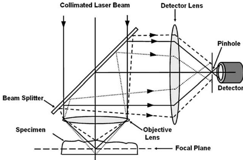
Fig. 2 Infinity-corrected confocal microscope.
