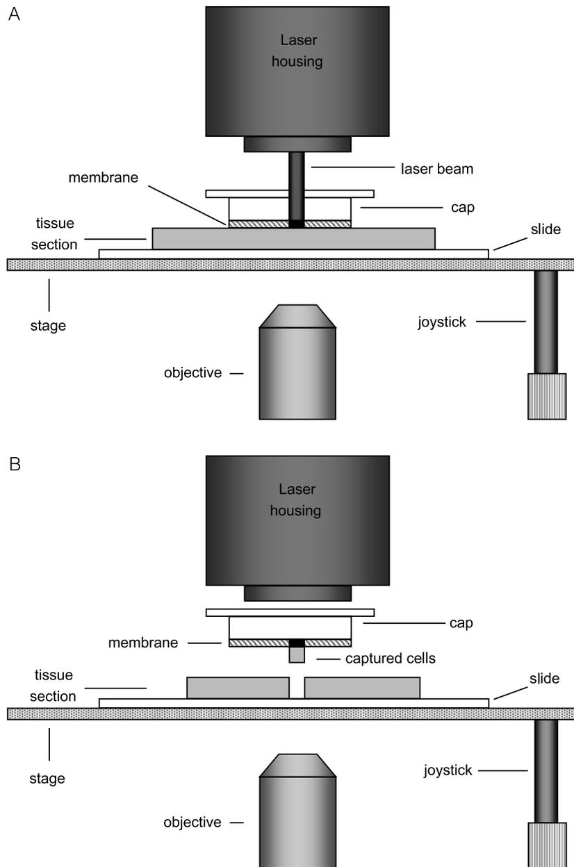
**Fig. 1** Schematic representation of laser capture microdissection. A) Activation of the laser leads to focal melting of the thermoplastic membrane attached to the lower portion of the optically transparent cap. B) Lifting of the cap leads to selective detachment of cells adherent to the molten (activated) parts of the membrane. (From Ref. [3].) (View this art in color at [www.dekker.com](http://www.dekker.com).)
