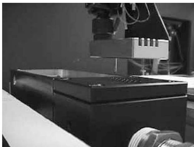
**Fig. 3** Experimental prototype of the DNA microarrayer: a close up view of a 32-pin dry station (Die-tech, San Jose, CA) that has been mounted to a specially designed wash station (Machine shop at HARC) secured to the base of the MicroLab 2200 between the two platforms. (View this art in color at [www.dekker.com](http://www.dekker.com).)
