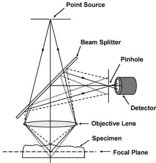
Fig. 1 Confocal laser microscope.
