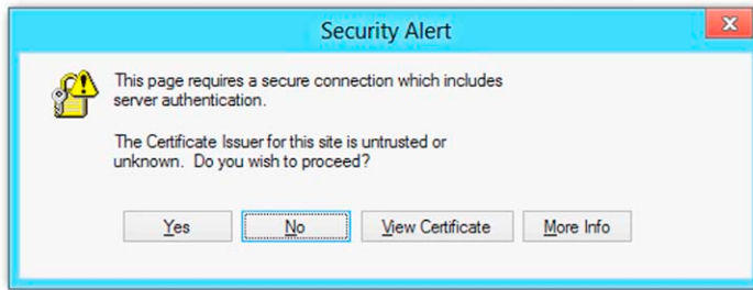
FIGURE 4.33 Security warning that appears when the certificate was issued by an untrusted CA.
