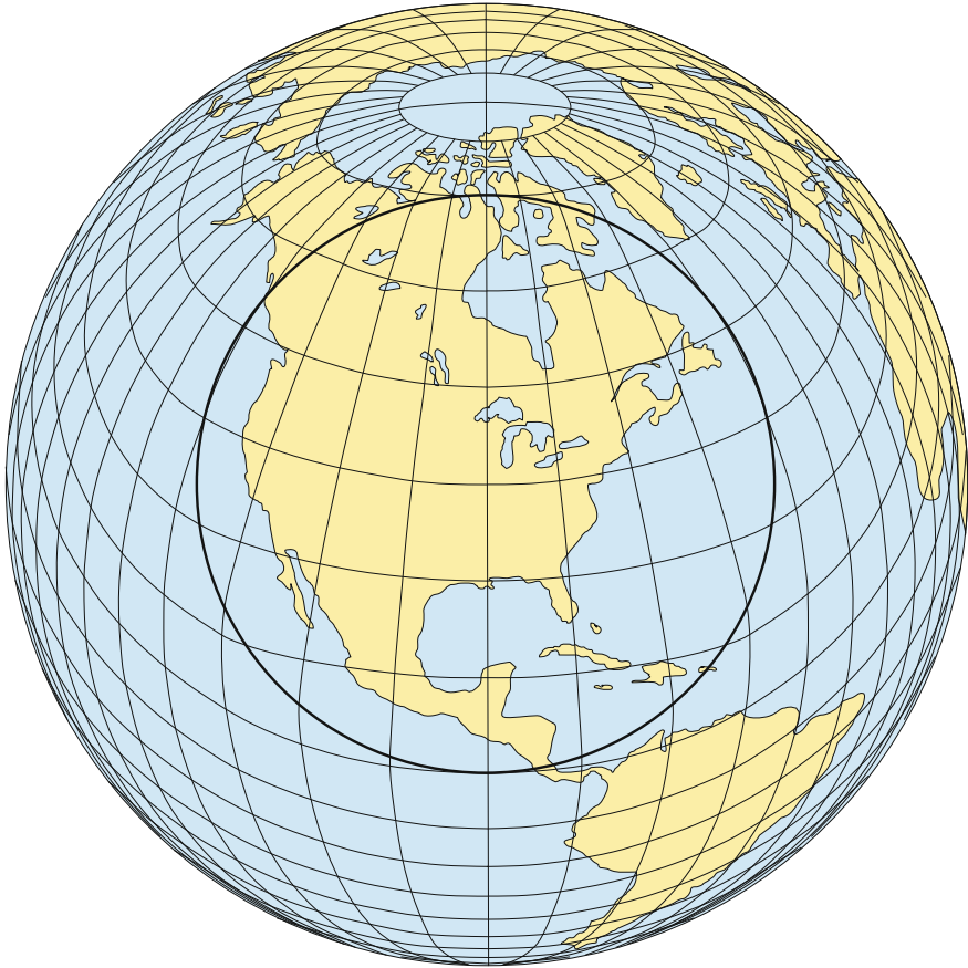
Fig. 3.38 A tapered “magnifying-glass” equal-area projection, with an inner circle 30^\circ in radius, and outer circle 120^\circ ; the radius of the inner circle is 0.65 that of the outer circle
