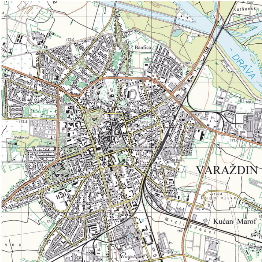
Fig. 12.20 Section of the topographic map in Gauss-Krüger projection, sheet Varaždin, 271-2-3, publisher: State Geodetic Administration of the Republic of Croatia, 1997, original scale 1:25,000
