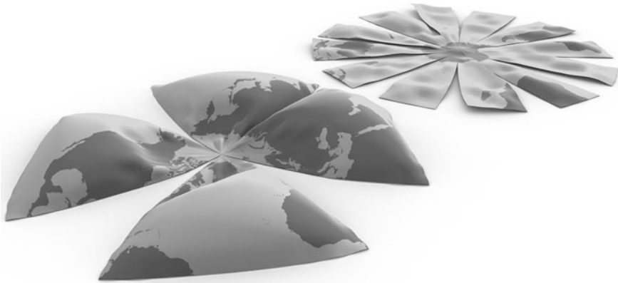
Fig. 9.1 The earth is impossible to unfold onto a planar surface without distortion
