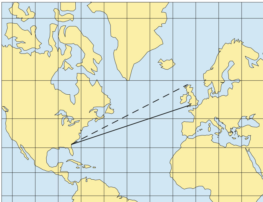
Fig. 3.59 A Mercator projection of the region in Fig. 3.58 with the correct rhumb. The dashed line shows where the “rhumb” on Fig. 3.58 would have led
