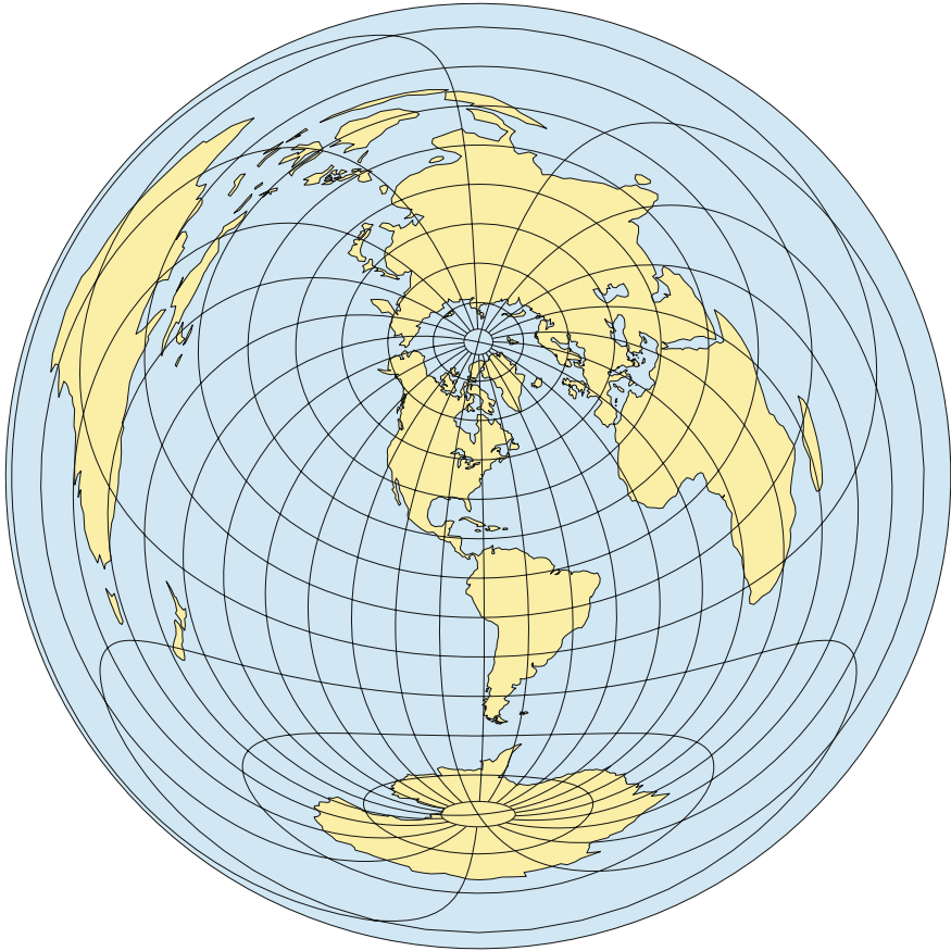
Fig. 3.60 The oblique azimuthal equidistant projection of the world centered on Washington, D.C
