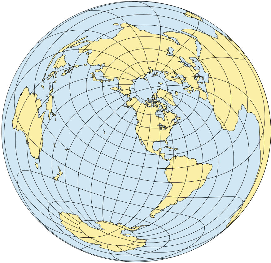
Fig. 3.65 The two-point equidistant projection of the world with centers at Washington, D.C., and Honolulu
