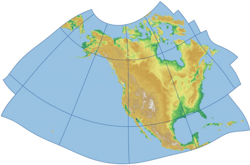
Fig. 12.51 GS50 projection encompassing the regions of the 50 states of the United States
