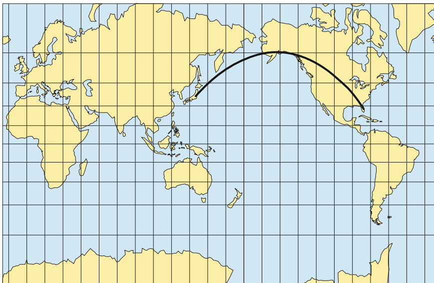
Fig. 3.54 The normal aspect of the Mercator projection showing the great circle between Miami and Tokyo
