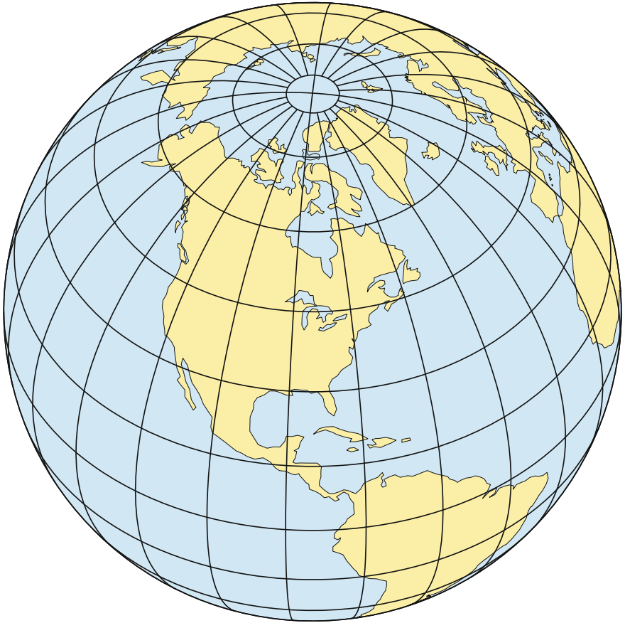
Fig. 3.34 The orthographic projection centered on the Great Lakes, 85^{\circ}\text{W} , 45^{\circ}\text{N} , as are Figs. 3.35, 3.36, 3.37 and 3.38
