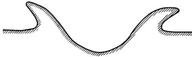
Figure 5.14 Section through a small-scale model in which the overturned flap is frozen. A section through the Vredefort impact structure exhibits such a flap.
