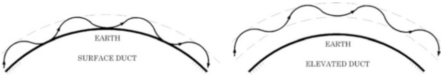
Fig. 3.6 Basic types of atmospheric ducts
