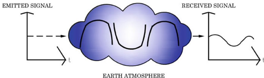
Fig. 9.2 Beam deviation due to large cells ( >\lambda )
